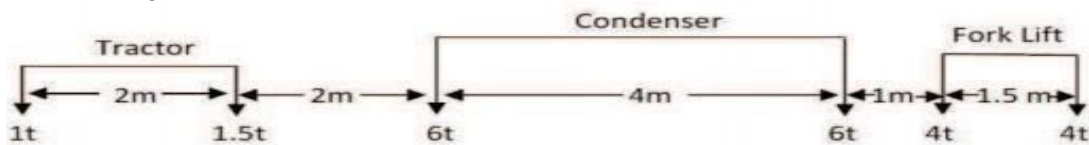
Loading on bridge deck during installation of Condenser.
