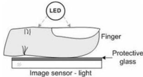
Fig. 3: Transmission Based Sensor
