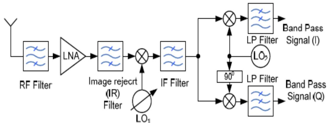
Fig. 1: Block Diagram of Heterodyne Architecture
