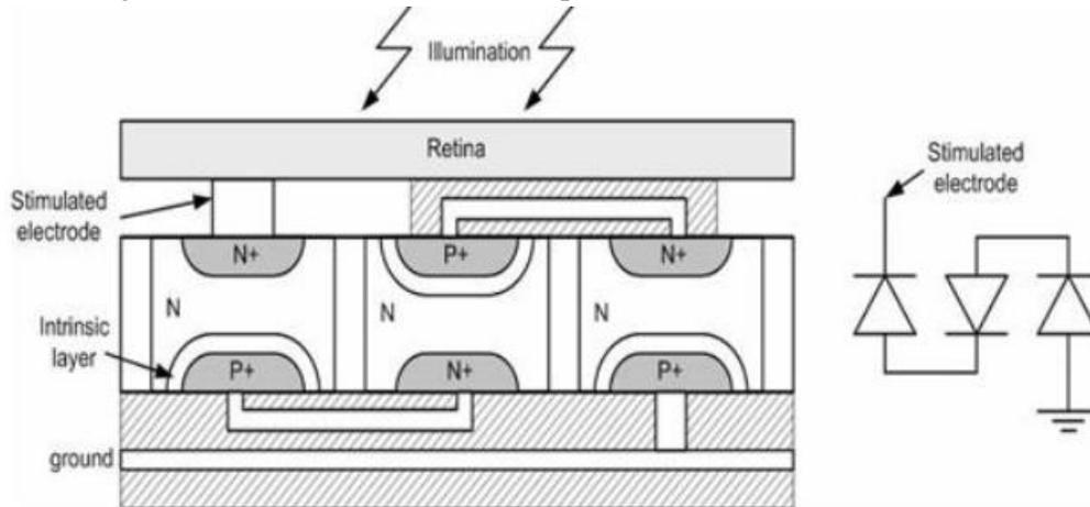
Fig. 5: Basic Architecture of Silicon Retina
