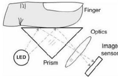
Fig. 2: Reflection Based Sensor
