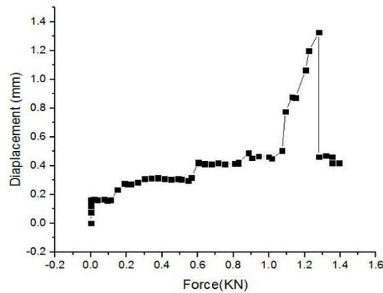
Fig.7 Tensile behavior of pure PLA
