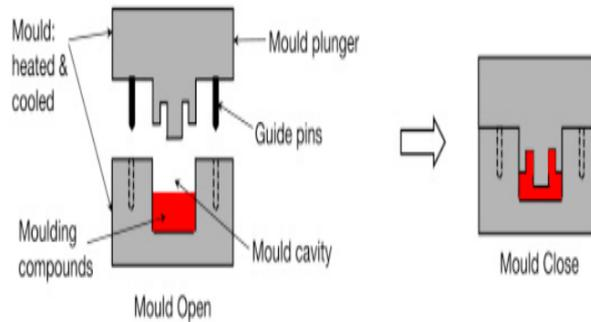
Fig.5 Compression molding machine setup
