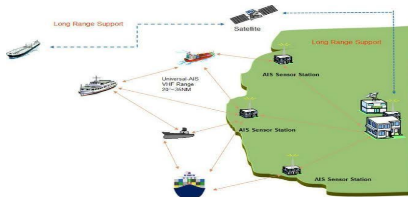
Figure 1. Diagram of AIS (Automatic Identification System)
