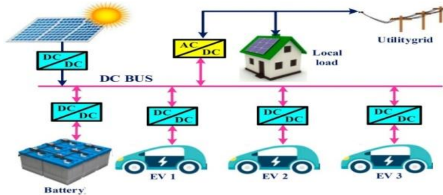
Figure 2 Proposed PV base Robotic Charging Station Model
