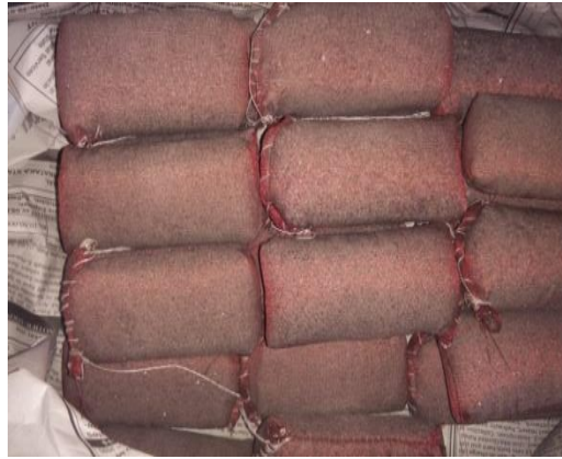
Figure 2: Geo textile bags filled with soil
