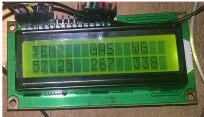
Figure 4: LCD showing output of Temperature, gas level and weight
