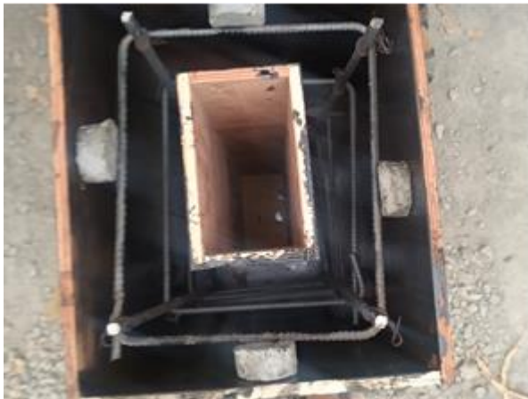
Fig.2. Mould of rectangular specimen
