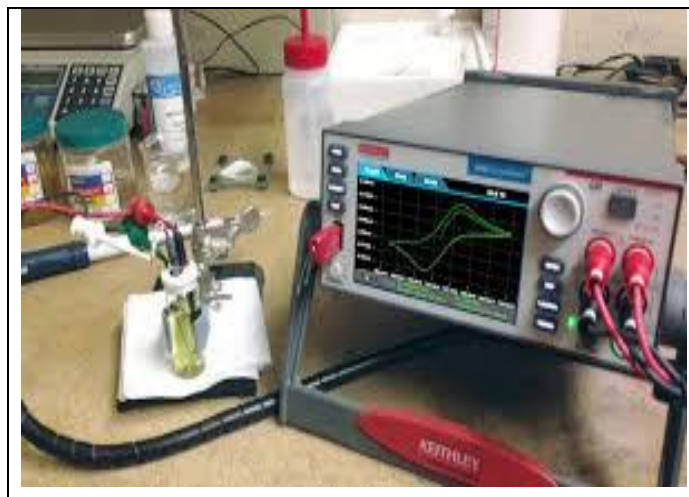
Figure 3: The biosensor cell with Re Dox output in E/H Software. The output is in the form of duck shape
