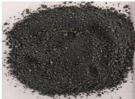
Fig.6 Copper Slag
