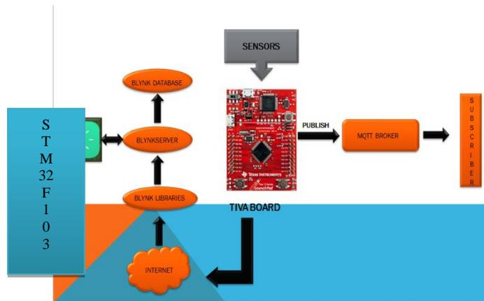
fig. 3. Block diagram of blynk controlled mqtt system
