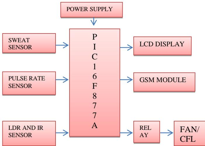
fig.1 Transmitter containing the sensors
