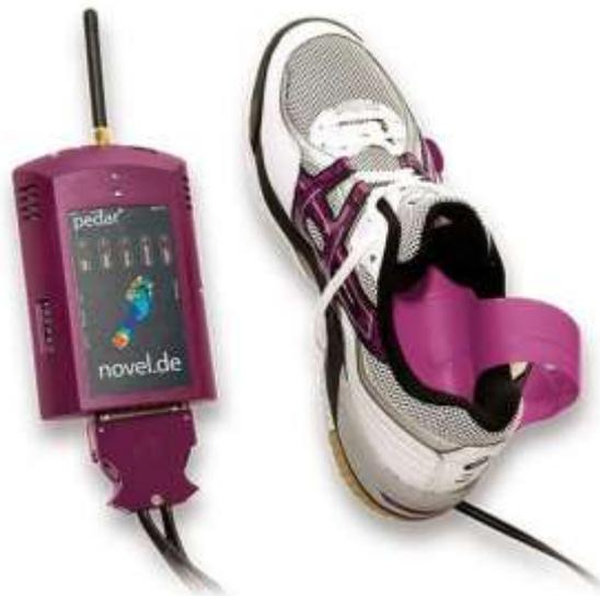
Fig. 5. In-shoe plantar pressure measurement system
