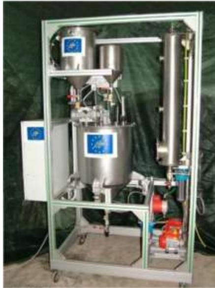
**Figure5: Pilot plant for biodiesel production [7]**
