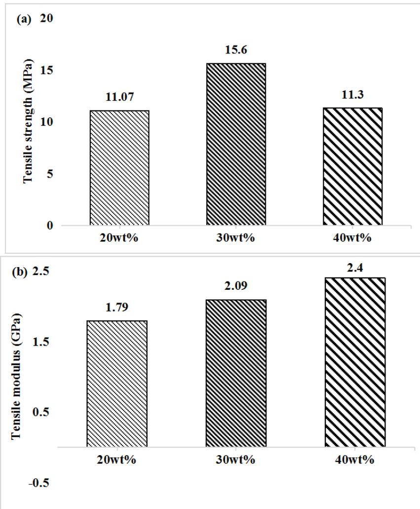
Fig. 4. Tensile properties of the various fiber loaded TFFRP composite samples, showing their tensile. (a) strengths and (b) moduli.
