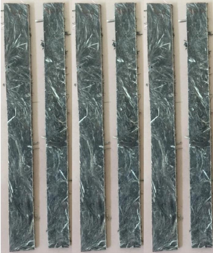
Fig. 3. TFFRP composite samples before tensile test.
