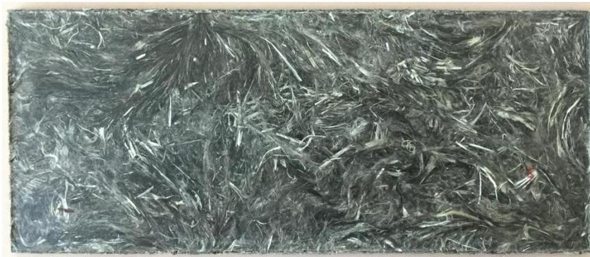
Fig. 2. Fabricated TFFRP composite plate.
