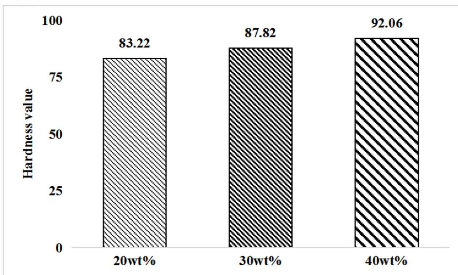
Fig. 5. Hardness value of the various fiber loaded TFFRP composite samples.
