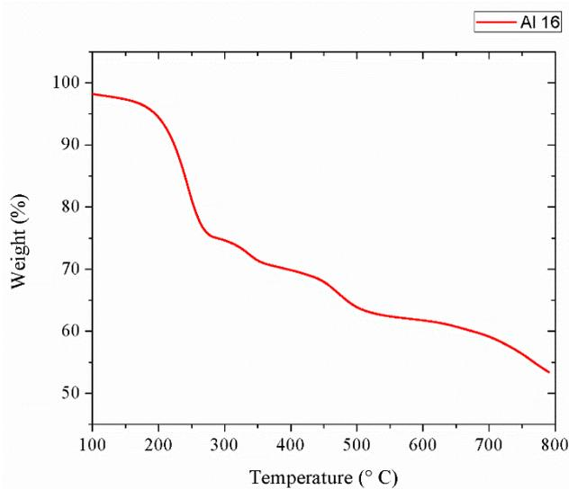
Fig.1(c) TGA for Al16 sample
