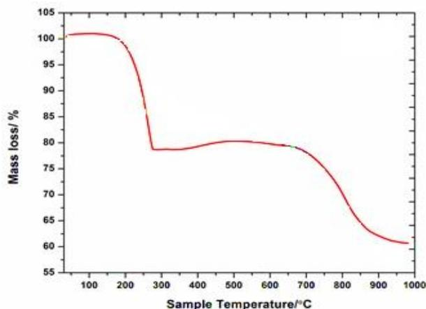
Fig.1(a) TGA for Normal firecracker sample
