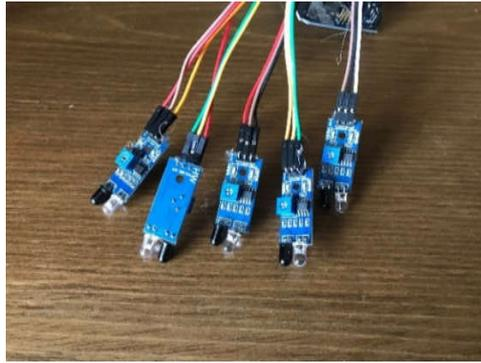
Fig. 5.16 Infrared (IR) Sensors
