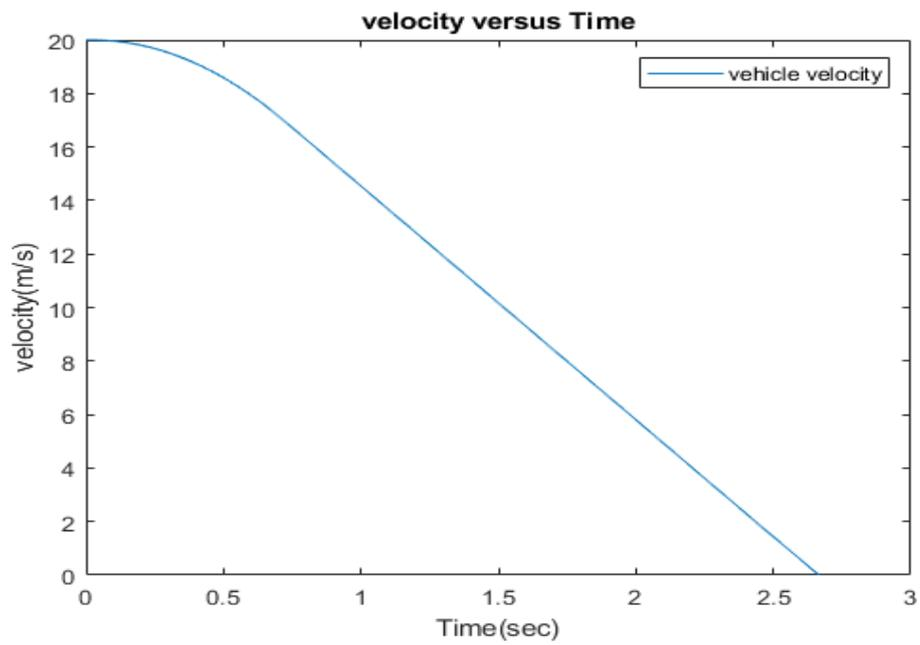
**Fig. 10** Vehicle speed versus time in vehicle braking using Bang-Bang controller.
