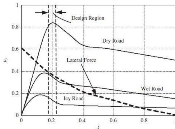
**Fig. 2 Road surface friction coefficient versus wheel slip ratio [5].**
