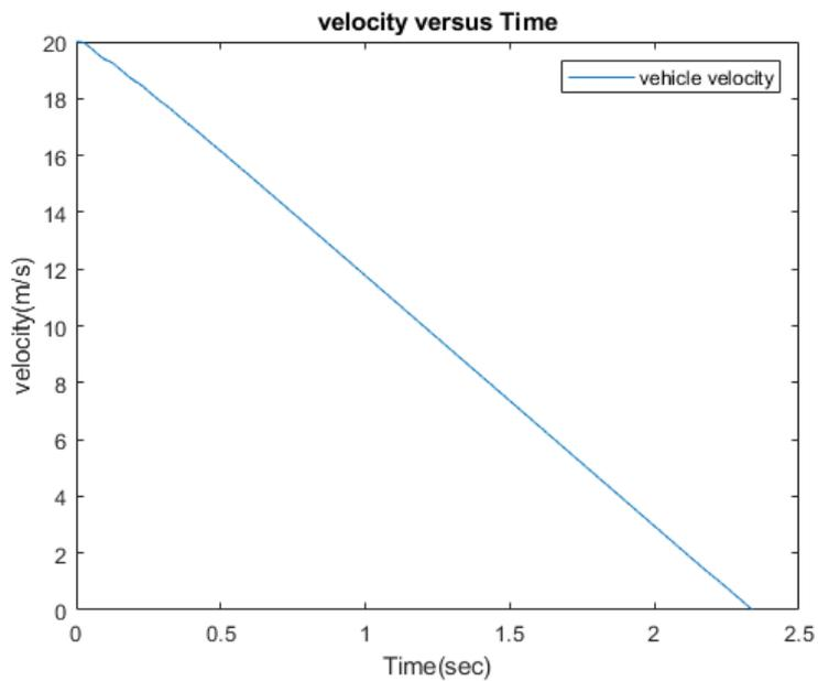
**Fig. 14 Vehicle speed versus time in vehicle braking using PD controller.**
