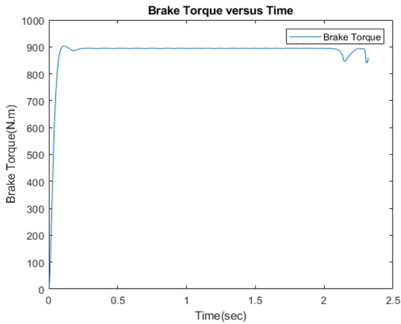
**Fig. 17 Braking torque versus time in vehicle braking using PID controller.**
