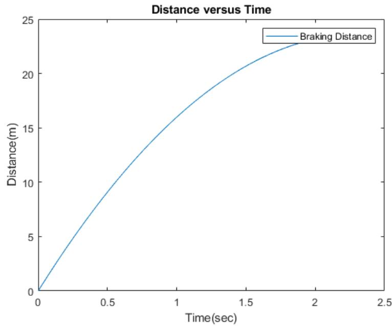
**Fig.19 Braking distance versus time in vehicle braking using PID controller.**
