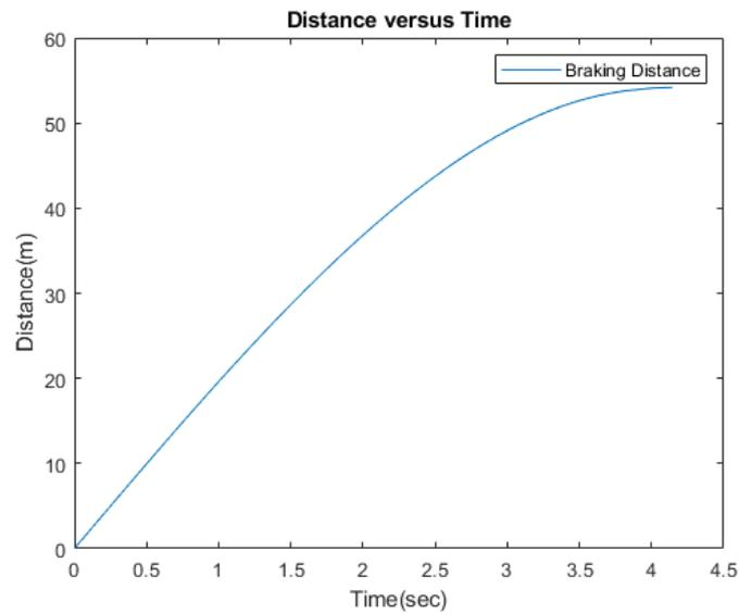
**Fig. 7 Stopping distance versus time in vehicle braking without controller**
