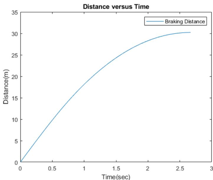
**Fig. 11 Braking distance versus time in vehicle braking using Bang-Bang controller.**
