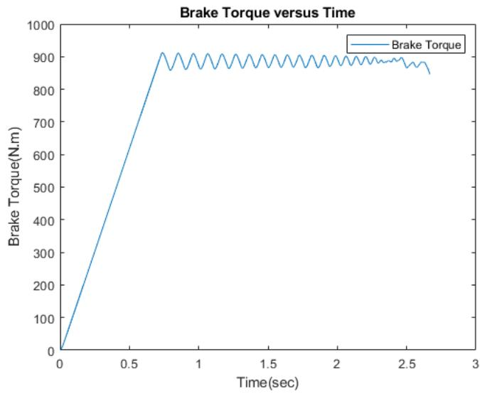
**Fig. 9** Brake torque versus time in vehicle braking using Bang-Bang controller.
