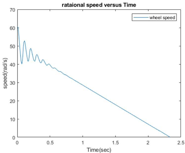
**Fig. 16 Wheel speed versus time in vehicle braking using PD controller.**
