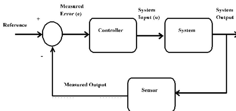
**Fig. 3 Block diagram of control system**
