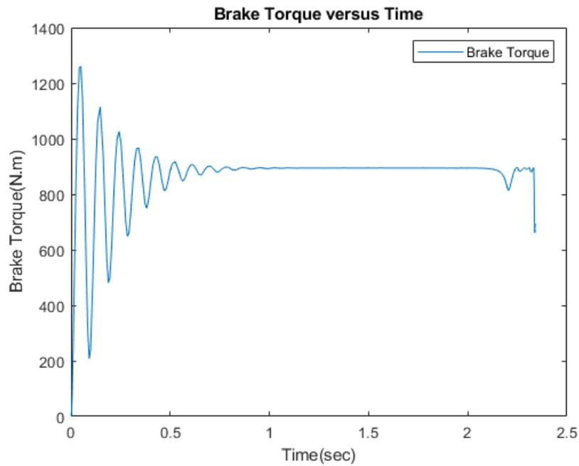
**Fig. 13 Brake torque versus time in vehicle braking using PD controller.**
