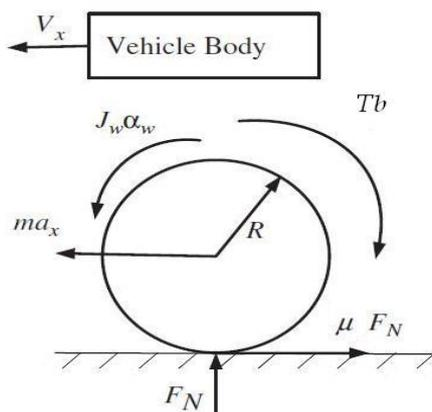
**Fig 1 Quarter car braking model**
