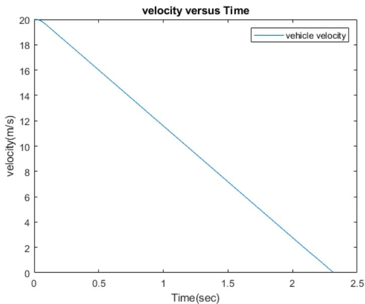
**Fig.18 Vehicle speed versus time in vehicle braking using PID controller.**
