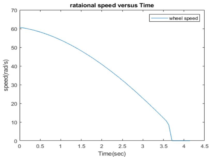
**Fig.8 Wheel rotational speed versus time in vehicle braking without controller.**
