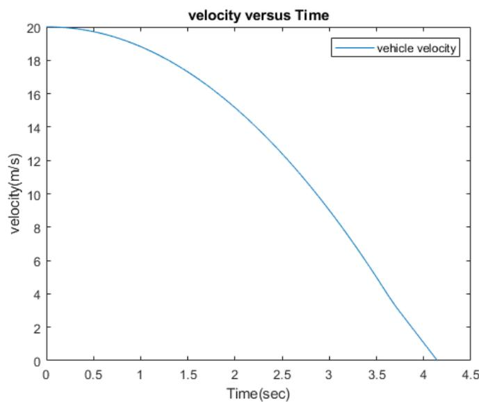
**Fig. 6 Vehicle speed versus time in vehicle braking without controller.**
