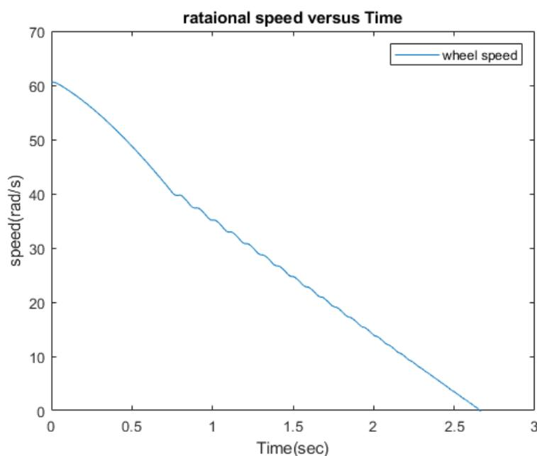
**Fig. 12 Wheel speed versus time in vehicle braking using Bang-Bang controller.**
