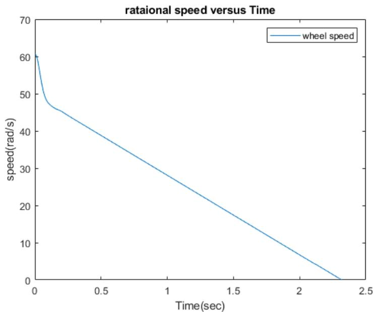
**Fig.20 Wheel rotational speed v/s time in vehicle braking using PID controller.**
