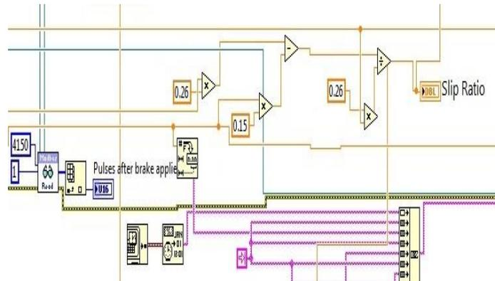
Figure-12. Calculating slip ratio in LabVIEW
