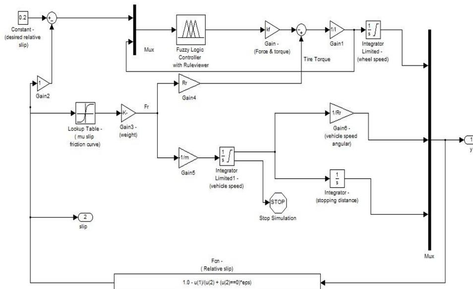
**Figure-10. ABS Simulink model for dry road conditions**
