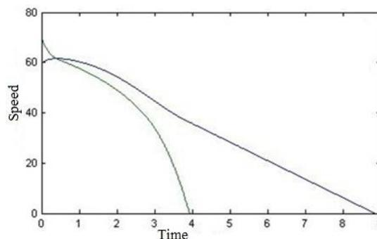
**Figure-17. Vehicle and wheel angular velocity without ABS**
