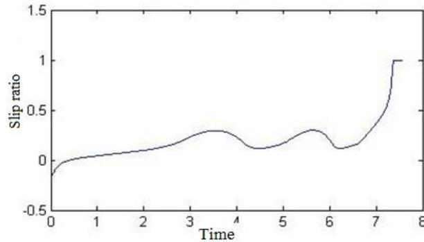
**Figure-18. Slip ratio for Fuzzy based ABS**
