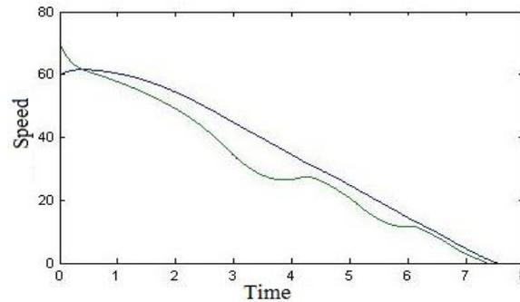
**Figure-16. Vehicle and wheel angular velocity with Fuzzy ABS**
