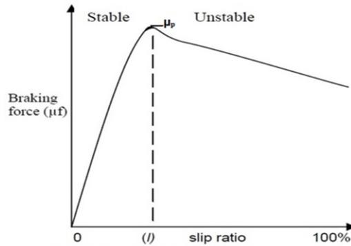
**Figure-2 Braking force and slip Relationship**
