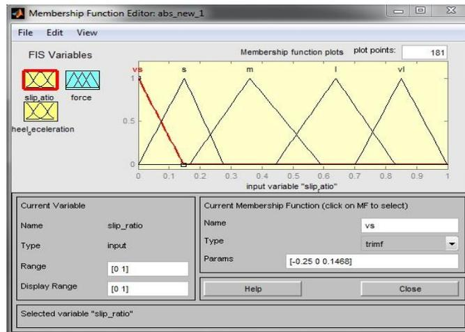
**Figure-4. Slip ratio representation in MATLAB**
