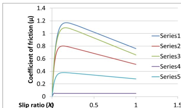
**Figure-1. Relationship between braking force and slip ratio for different road surfaces.**
