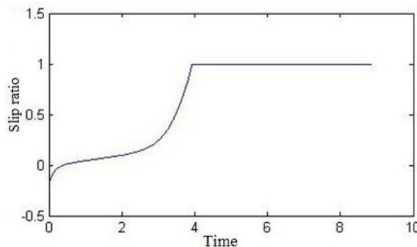
**Figure-19. Slip ratio for system without ABS**
