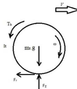
**Figure-3 Braking condition free body diagram of wheel**
