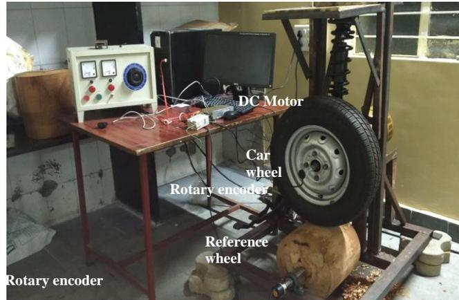
**Figure-11. Experimental Setup**
