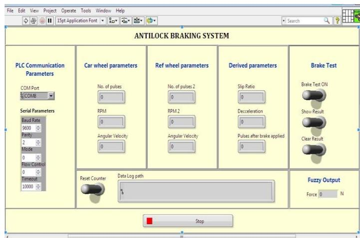
**Figure-15. Virtual Interface for ABS**
