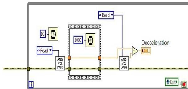
Figure-13. Wheel deceleration calculation in LabVIEW
