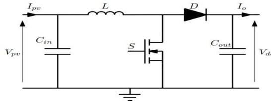
Fig.4: DC-DC Boost Converter
