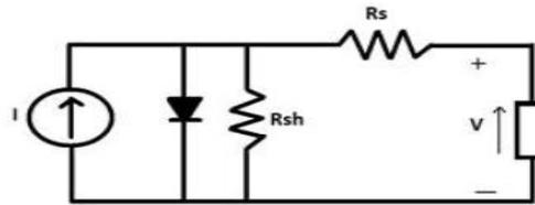
Fig.2: Equivalent Circuit of solar cell
