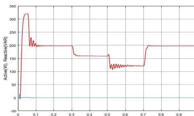
Fig. 8: MFO grid power in high irradiation variation.
