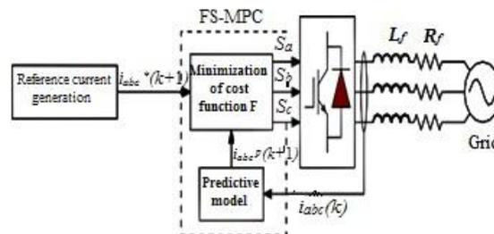
Fig. 3: Predictive current control for VSI and the grid
