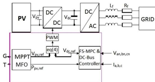
Fig.1: Block diagram of the PV array with MPPT and grid-connected system.
