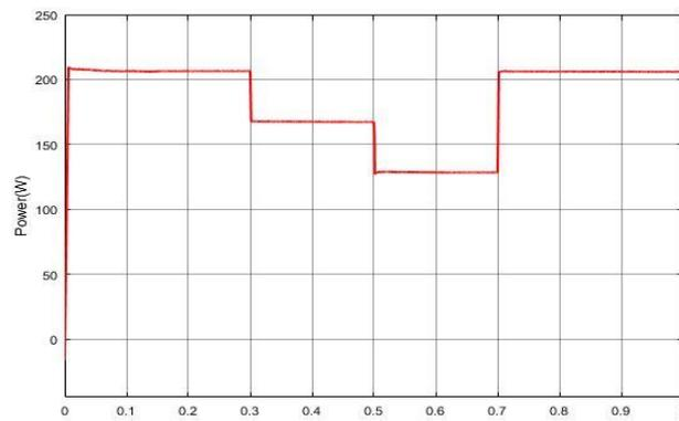
Fig. 5: Power of MFO MPPT algorithm as transferred to grid
