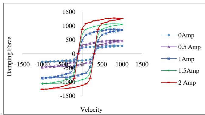
Figure 20: Damping Force Vs Velocity Plot at different current input for MR4
