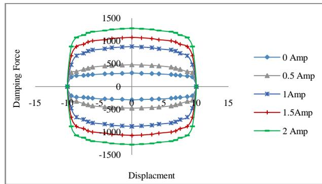
Fig 19: Damping Force Vs Displacement Plot at different current input for MR4
