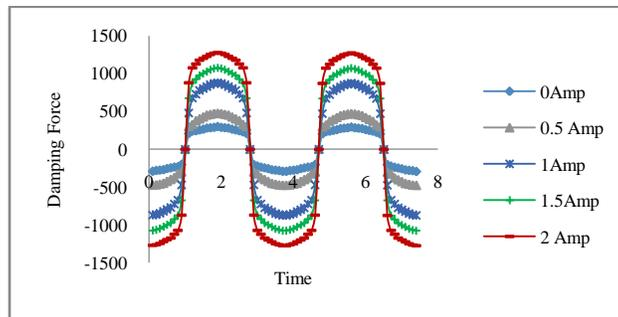
Figure 18: Damping Force Vs Time Plot at different current input for MR4
