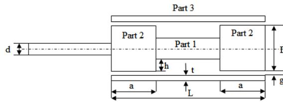
Fig 6: Piston with groove
