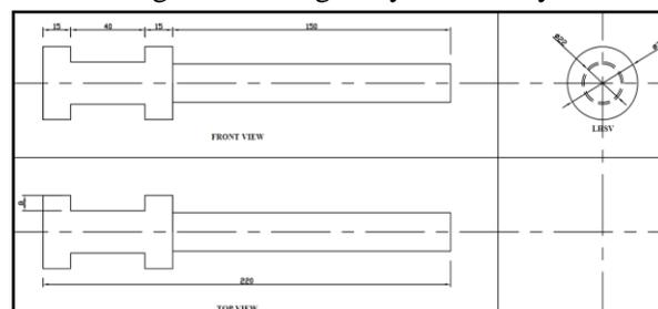
Fig. 4: Drawing of Piston body
