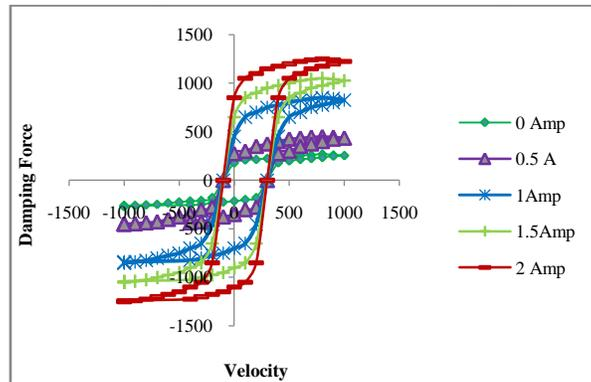
Fig 14: Damping Force Vs Velocity Plot at different current input for MR1
