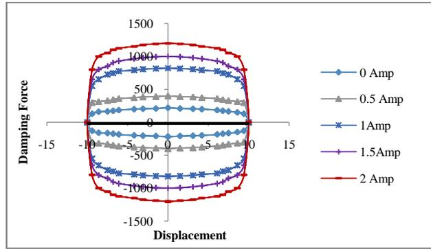
Figure 16: Damping Force Vs Displacement Plot at different current input for MR3
