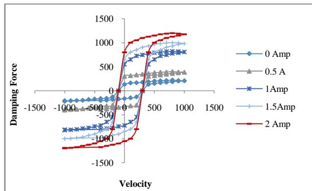
Figure 17: Damping Force Vs Velocity Plot at different current input for MR3
