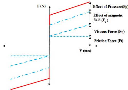
Fig: 5: The total damping force of MR damper is sum of: friction force, viscous force, controlling force and pressure driven force.
