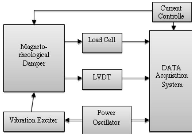
Fig 10: Layout of Experimental Set-up
