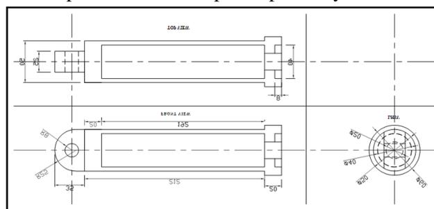
Fig. 3: Drawing of cylinder body
