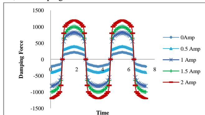
Fig 15: Damping Force Vs Time Plot at different current input for MR3
