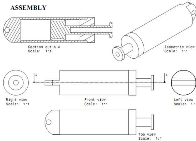
Fig 9: Assembly Drawing of MR damper
