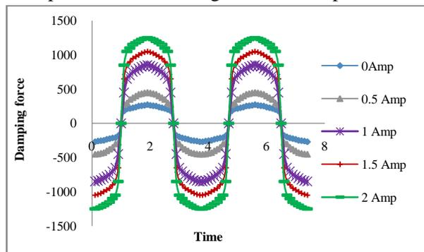
Fig 12: Damping force Vs Time for MR1 sample at different current input
