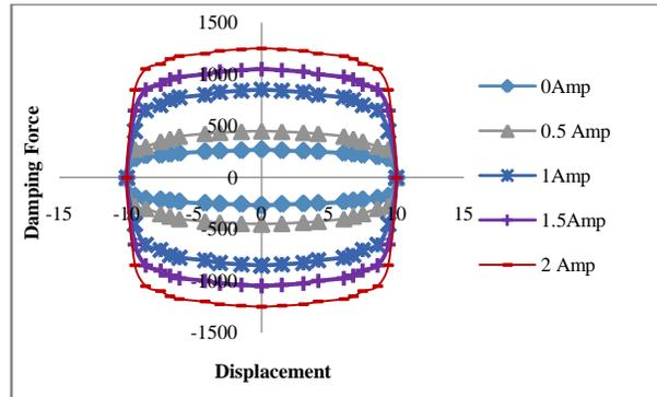
Fig 13: Damping Force Vs Displacement Plot at different current input for MR1
