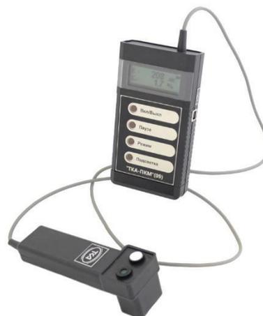
Figure 2. A measuring instrument used in the study to determine level of natural and artificial illuminance
