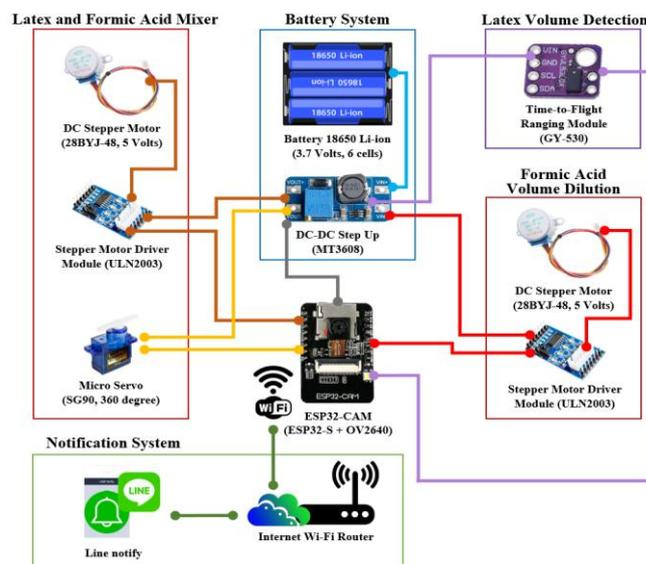
**Figure 2. All Electronic Devices and Sensors based on IoT for Improving the Rubber Cup Lump Production**
