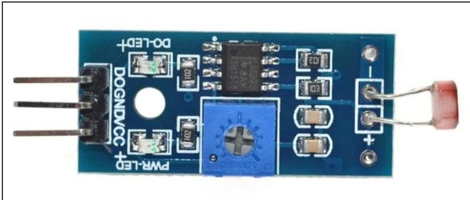
Fig 3.3 LDR sensor module
