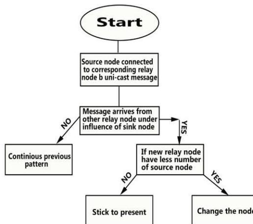
Figure 4: Procedural diagram of step #4 (selecting the relay node as parent node depending on repetitive controlled algorithm)
