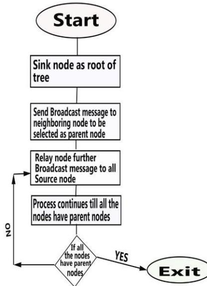
Figure 3: Procedural diagram of step #2 and 3 (selecting the relay node as parent node by the source node)
