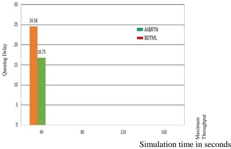
Figure 7: Comparison of AIBRTN with BDTML in term of Queuing Delay
