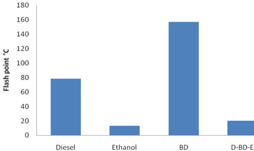
**Fig 6.4** Flash point of different test fuels
