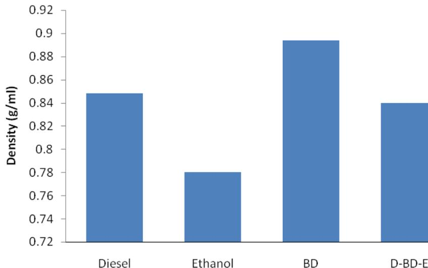
**Fig. 6.1** Density of different test fuel samples
