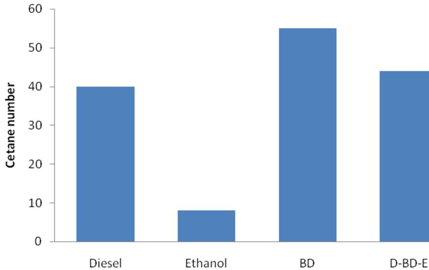
**Fig. 6.5** Cetane number of different test samples
