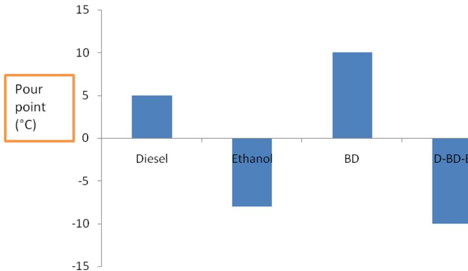
**Fig. 6.6** Pour point of different test fuel samples
