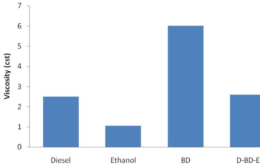
**Fig. 6.2** Kinematic viscosity of test fuel samples
