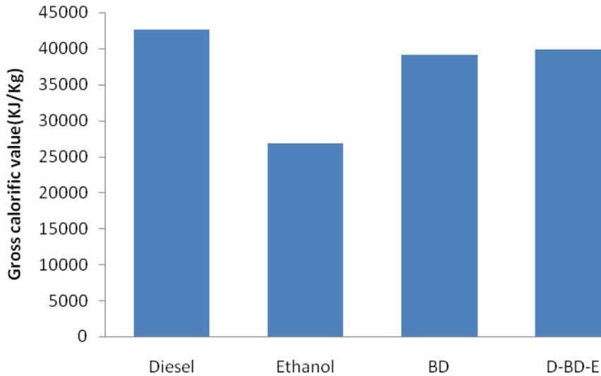
**Fig. 6.3** Gross calorific values of test fuels
