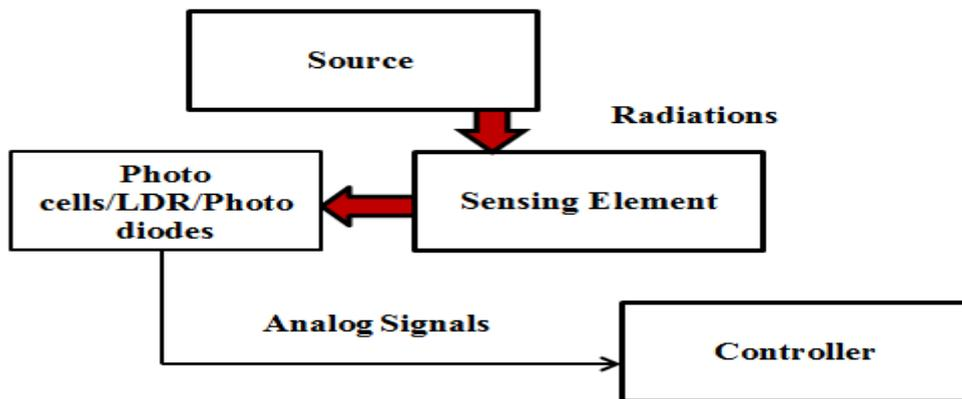
**Figure 2: Components for design and characterization of solar sensors**
