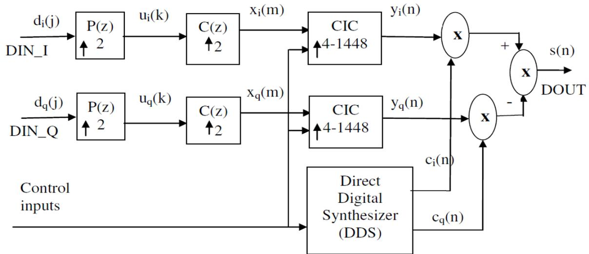
**Figure 3.1 Block diagram of Digital Up Converter (DUC)**
