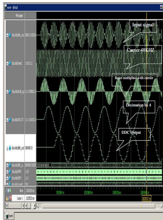
**Figure 5.4 ModelSim Simulation result of DDC.**
