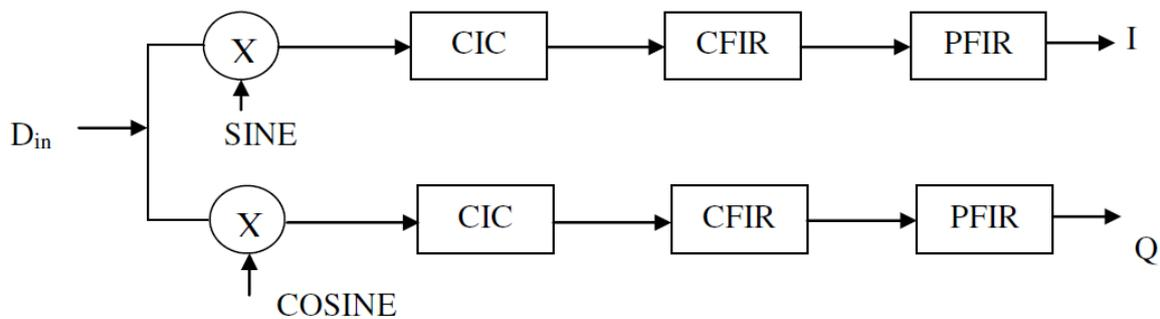
**Figure 3.2 Block diagram of Digital Down Converter (DDC)**
