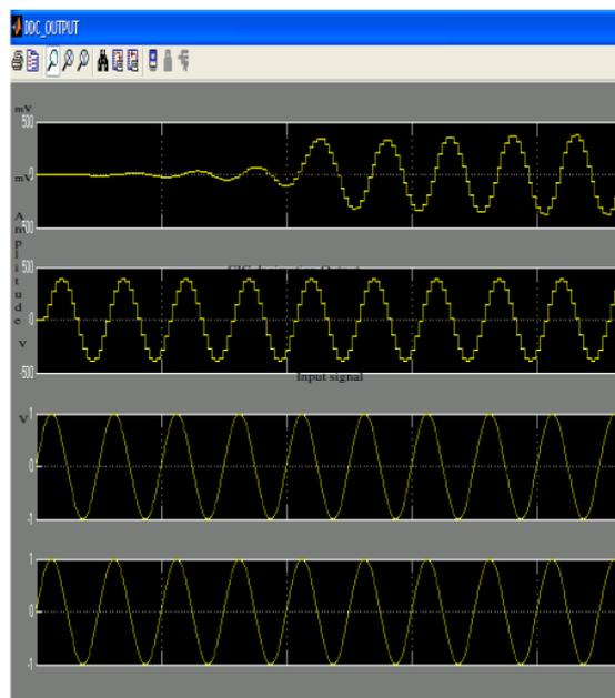
Figure 5.2 MATLAB simulation result of DDC in time-domain.
