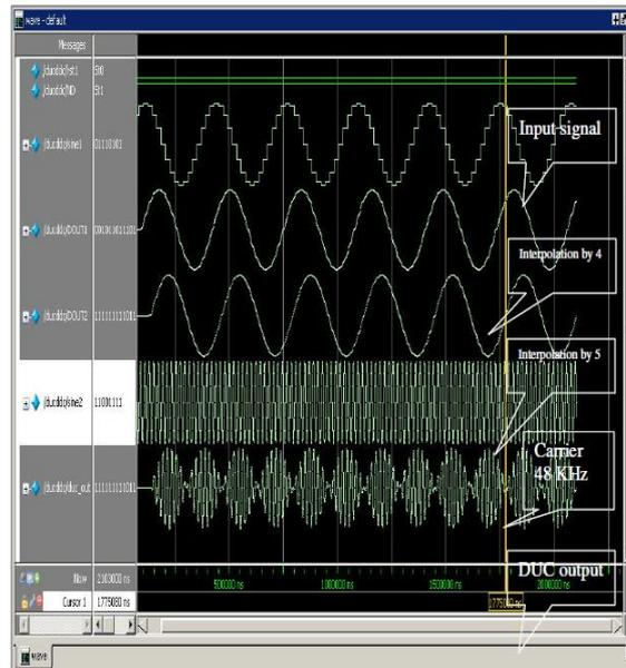
**Figure 5.3 ModelSim Simulation result of DUC.**
