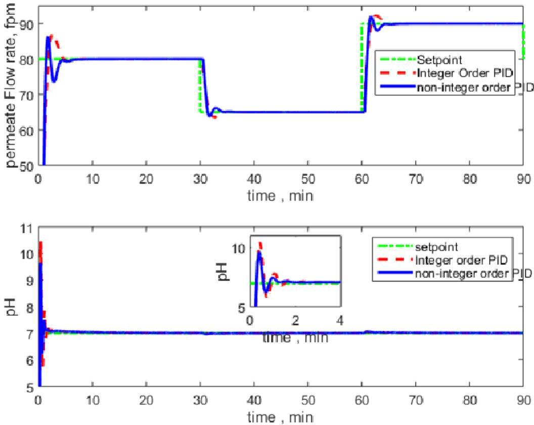
Fig.8. Servo and regulatory response of multiloop IMC-PID controller
