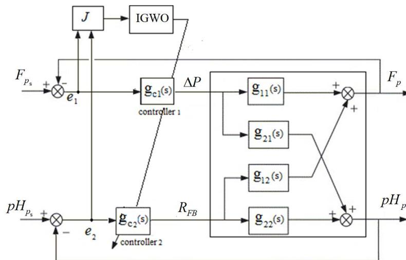
Fig 6. The Improved GWO based Multiloop non-integer order PID controller tuning.
