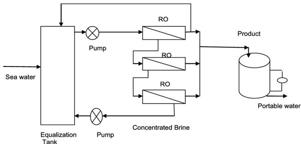
Fig.2. Schematic diagram of Reverse osmosis process
