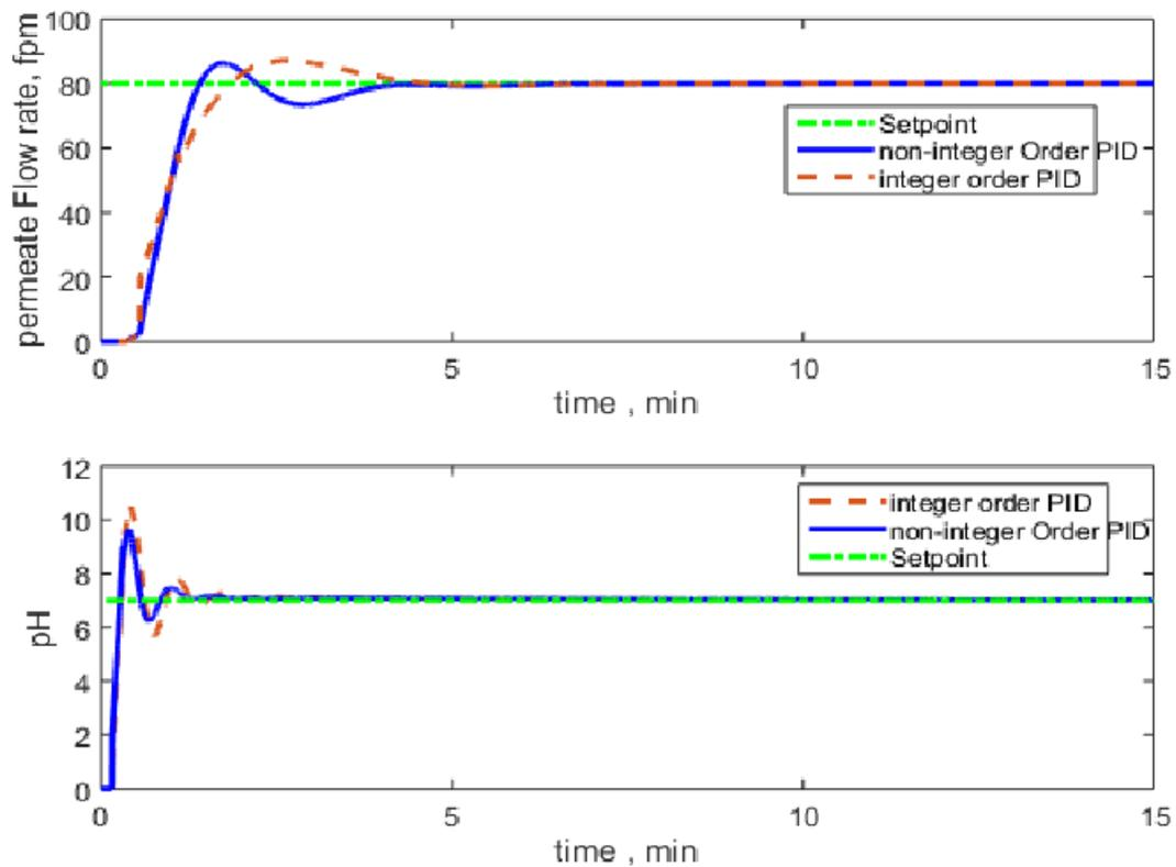
Fig.7. Servo response of multiloop IMC-PID controller
