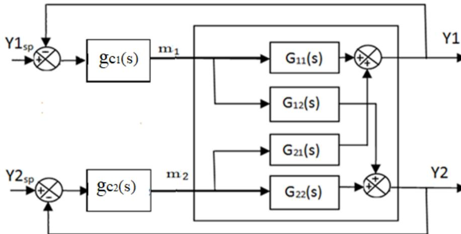
Fig.3 Multiloop control scheme
