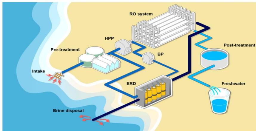
Figure 1. Sea Water Reverse Osmosis Desalination Process [17]
