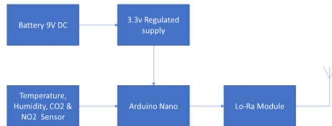
**Fig 1: Transmitter block**
