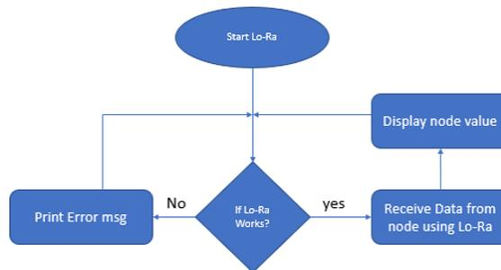
**Fig 4: Flow chart of receiver System**
