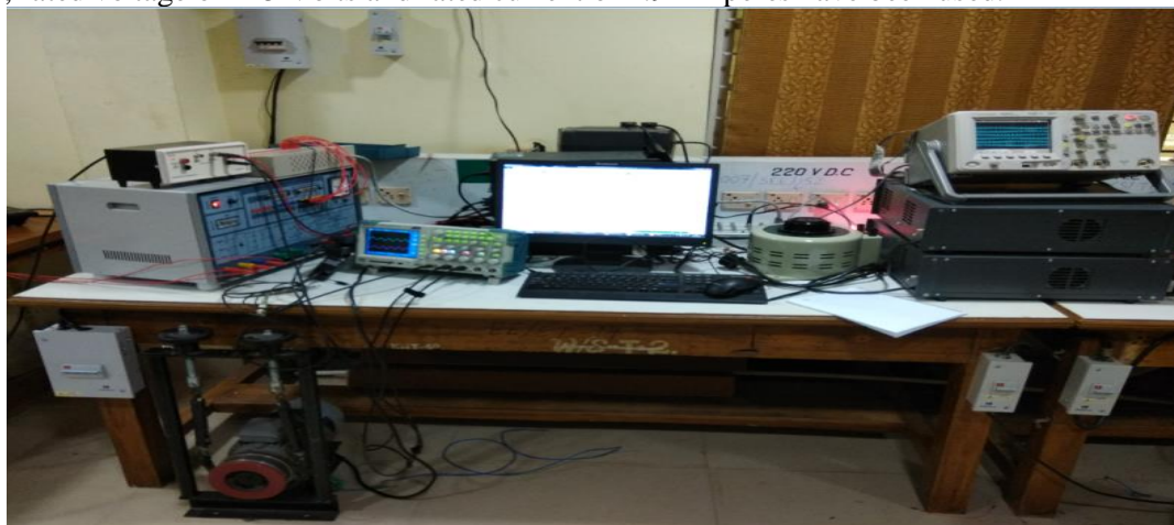
Fig. 2. Experimental Setup to generate the induction motor parameters.
