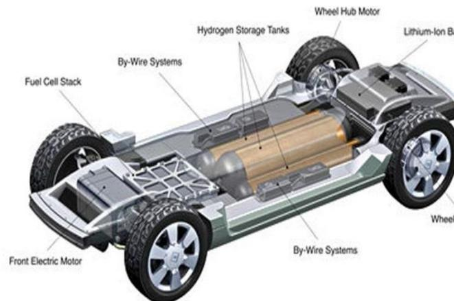
Figure 1. Schematic view of hydrogen-wire car
