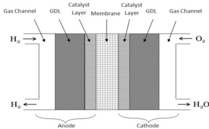
**Figure 1. Components of Fuel Cells**
