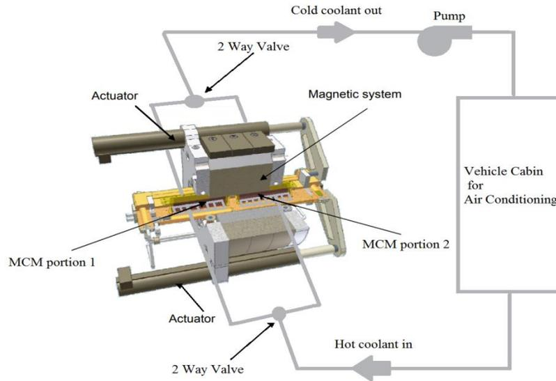
**Figure 2. Magneto-caloric air conditioning design**
