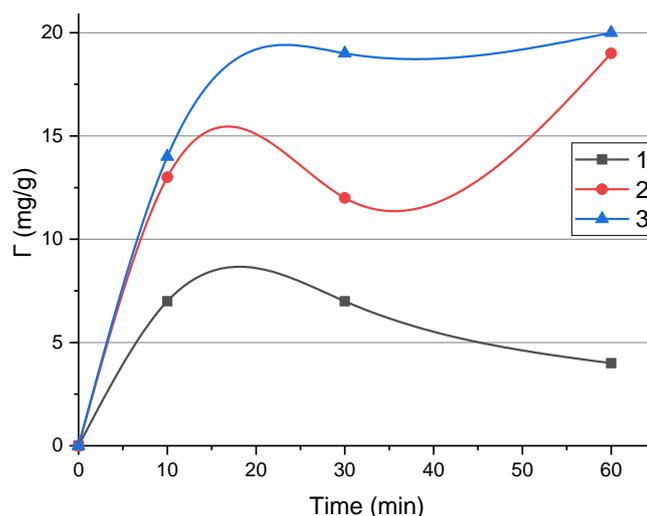
**Figure 5. Kinetic curve of sorbents to carbon dioxide, where: 1-natural bentonite; 2- high-silicon zeolite bentonite treated with a 1% solution of hydrochloric acid and sodium carbonate; 3 - high-silicon zeolite bentonite treated with a 10% solution of sulfuric acid and sodium carbonate.**
