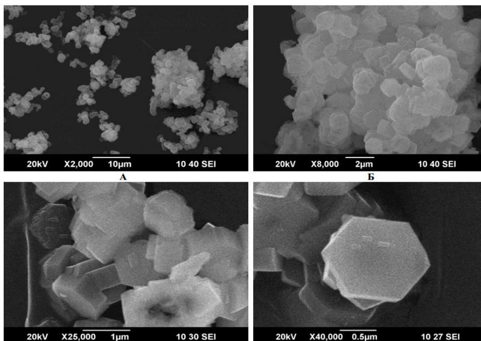
**Figure 1. Microphotograph of HSZ obtained in scanning electron microscope: (up) (A)  $\times 2000$  magnification; (B)  $\times 8000$  magnification; (bottom) (A)  $\times 25000$  magnification; (B)  $\times 40000$  magnification.**
