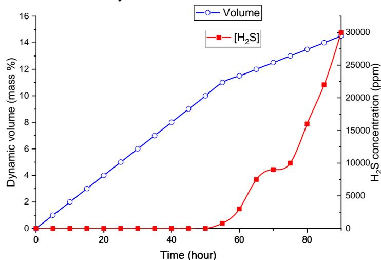
**Figure 4. Changes in the dynamic capacity of the chemisorbent  $\text{CaCl}_2 \cdot \text{ZnCl}_2 \cdot \text{MnCl}_2/\text{HSZ}$  at the outlet of the adsorber with time.**
