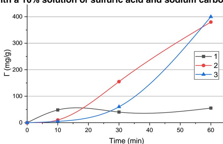
**Figure 6. Kinetic curve of sorbents to hydrogen sulfide, where: 1- natural bentonite; 2- high-silicon zeolite bentonite treated with a 1% solution of hydrochloric acid and sodium carbonate; 3 - high-silicon zeolite bentonite treated with a 10% solution of sulfuric acid and sodium carbonate.**
