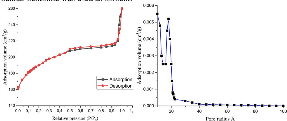
**Figure 2. Adsorption-desorption isotherms and pore size distribution differential curves related to radius of synthesized sorbents.**
