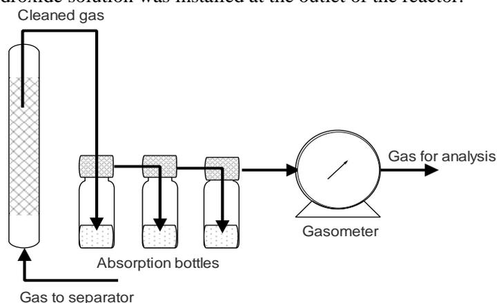
**Figure 3. Experimental adsorber device for the purification of petroleum gases from hydrogen sulfide.**
