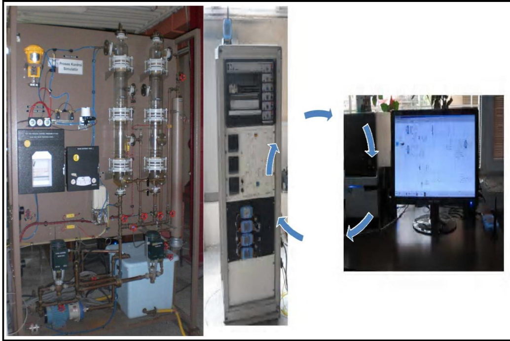
Figure 1. Experimental system: Process simulator, control panel and computer on-line connected to simulator with wireless technology
