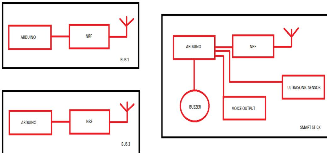
**Fig. 4. Block diagram of proposed system (Transmitter and Receiver)**
