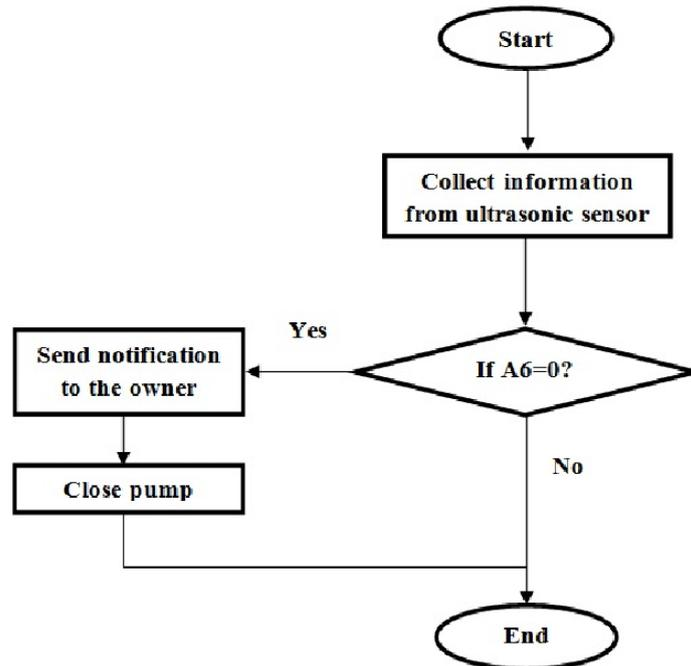
Fig.6. Ultrasonic loop diagram
