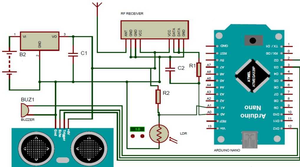
Fig. 5. Obstacles detection pin diagram
