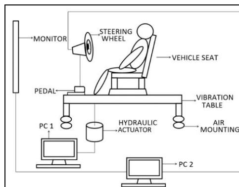
Figure 1. Schematic drawing of the experiment setup. An actual vehicle's seat was mounted on a vibration table. A hydraulic actuator located at the corner of the table will provide multi-axial input to the volunteer. A simulator also consists of a personal computer, a monitor and peripheral steering wheel, accelerator, and brake accessories.
