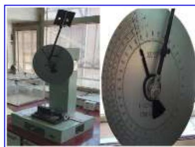
Fig. (5) Impact Test
