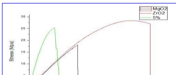
Figure (9) the tensile stress-strain curve of compound materials by nanoparticle's type.
