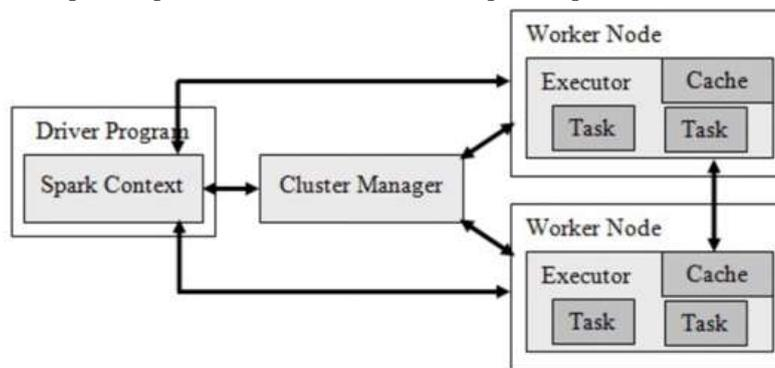
**Figure 5: Architecture of Apache Spark**
