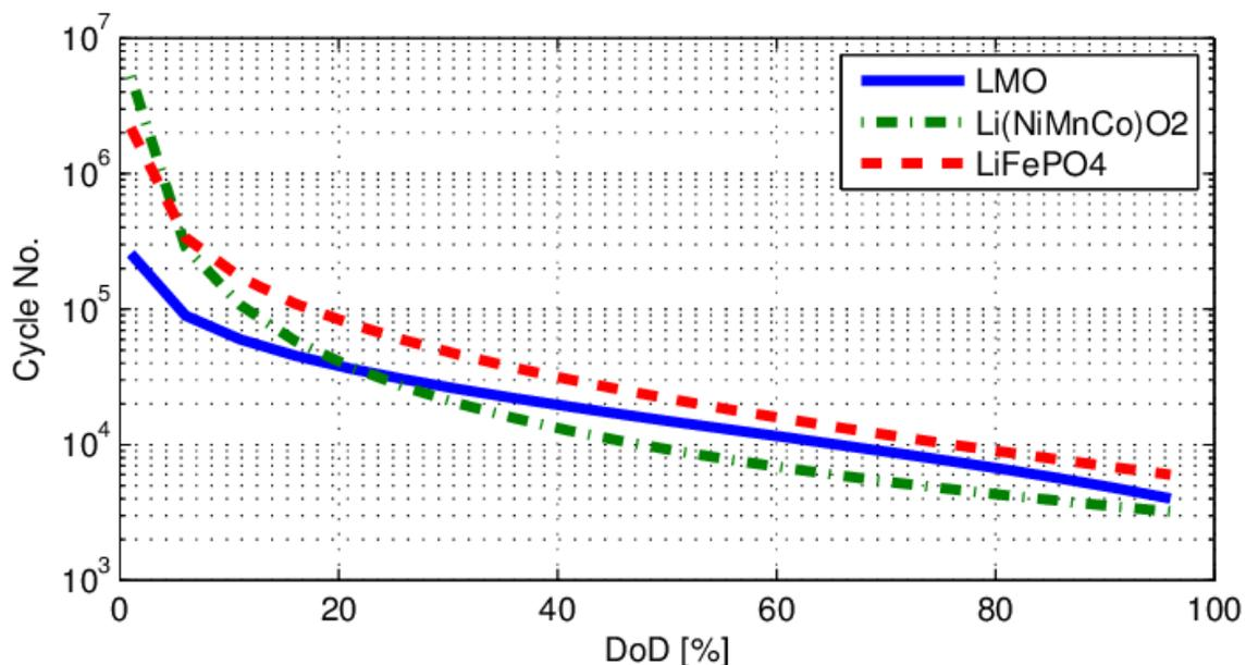
In the above graph, it can be seen that LiFePO<sub>4</sub> cells have more charge discharge cycle than other lithium chemistry cells. If proper care is taken then and battery is charged after 80% DOD then battery would last more than 2000 charge discharge cycle.
