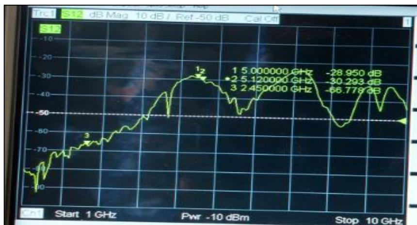
**Figure 17 . Mutual coupling for DSCSRR structure in ground**
