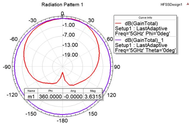
**Figure 4: Radiation Pattern of Simple Coplanar 2 X 2 Microstrip Array Antenna**
