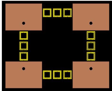
Fig 6: Top view of the four patch antennas with CSRR etched on ground plane.
