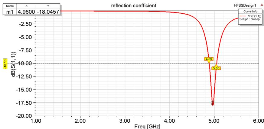
**Figure 7: S11 of Coplanar 2 X 2 Microstrip Patch Array Antenna with SRR**
