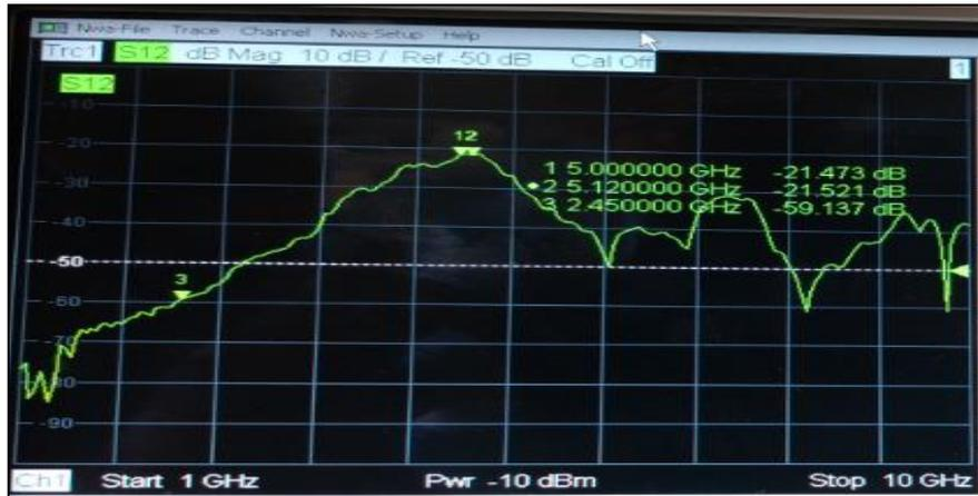
**Figure 16. Mutual Coupling For SRR structure in ground**
