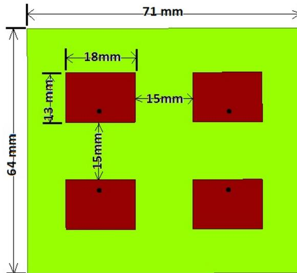
Figure 2: Simple Coplanar 2 X 2 Microstrip Array Antenna
