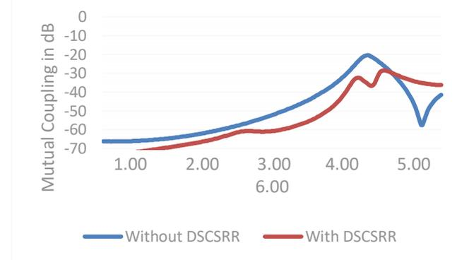
**Figure 12. Mutual coupling between four patch antennas with and without CSRR**
