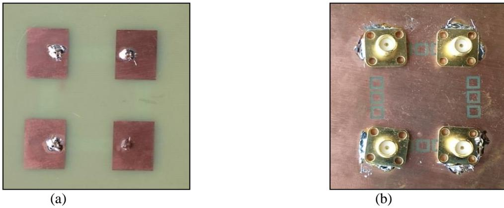
**Figure 14. Fabricated antenna (a) Top view (b) Bottom view**
