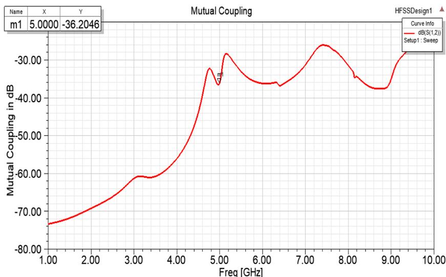
**Figure 10. Mutual Coupling of Coplanar 2 X 2 Microstrip Patch Array Antenna with DSCSRR**
