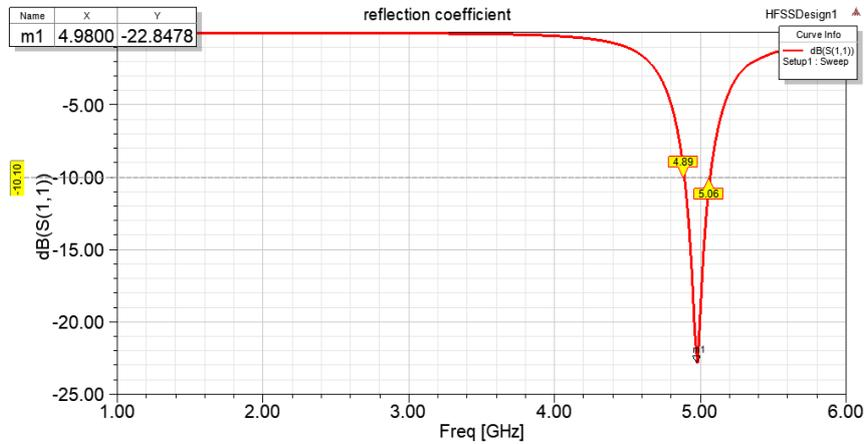
**Figure 9. S11 of Coplanar 2 X 2 Microstrip Patch Array Antenna with DSCSRR**
