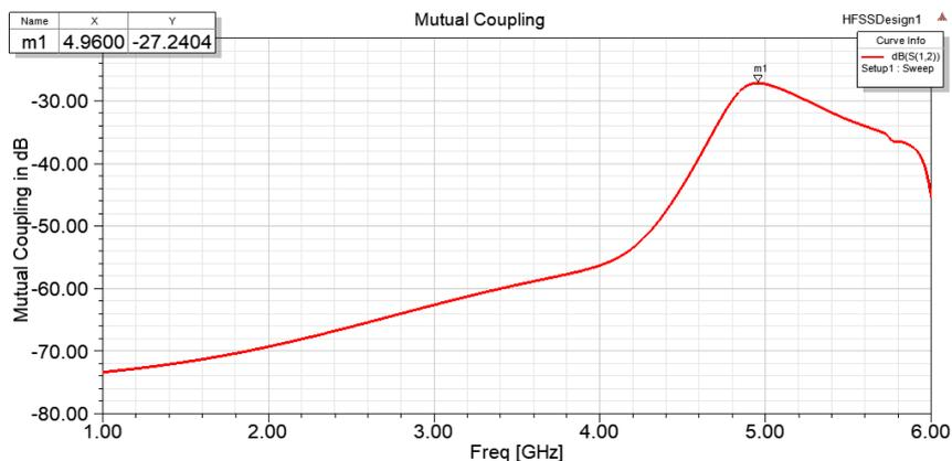
**Figure 8. Mutual Coupling of Coplanar 2 X 2 Microstrip Patch Array Antenna with SRR**
