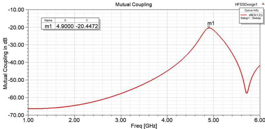
**Figure 5: Mutual Coupling of Simple Coplanar 2 X 2 Microstrip Array Antenna**
