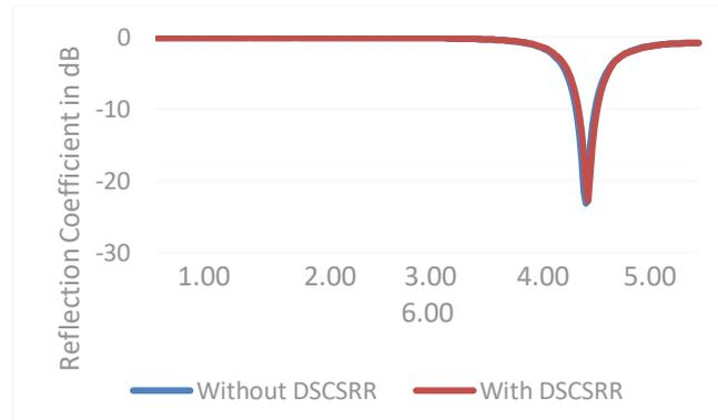
**Figure 11. Return loss (S11) of four patch with CSRR and without CSRR**
