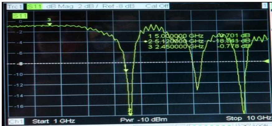
**Figure15. Reflection Coefficient observed on VNA**
