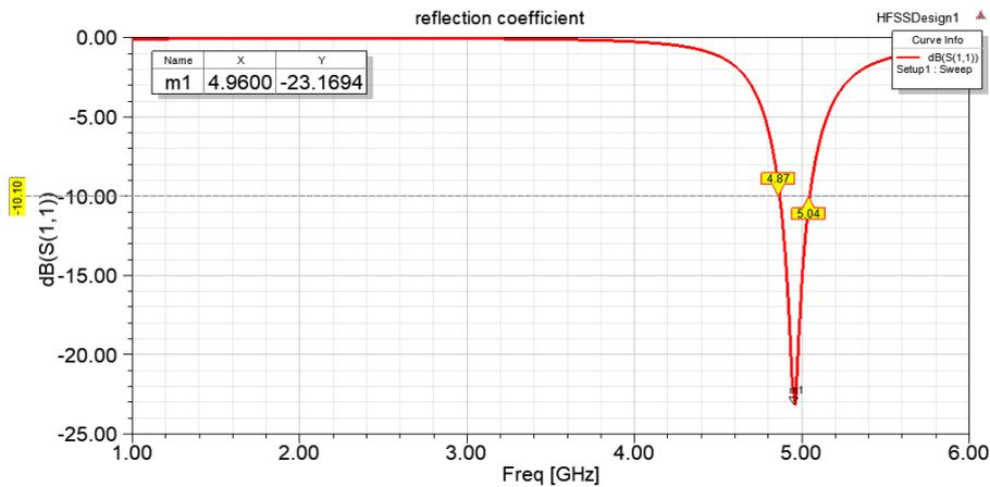
Figure 3:  $S_{11}$  of Simple Coplanar 2 X 2 Microstrip Array Antenna
