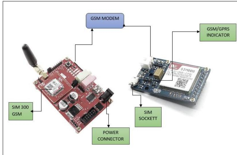
**Figure 3. Image of GSM Modem circuit**
