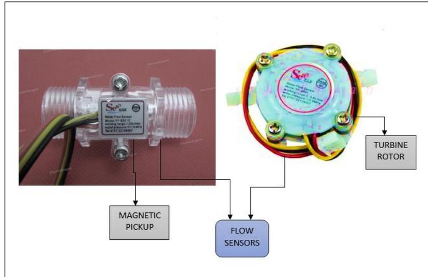
Figure 4. Image of Water Flow Sensor
