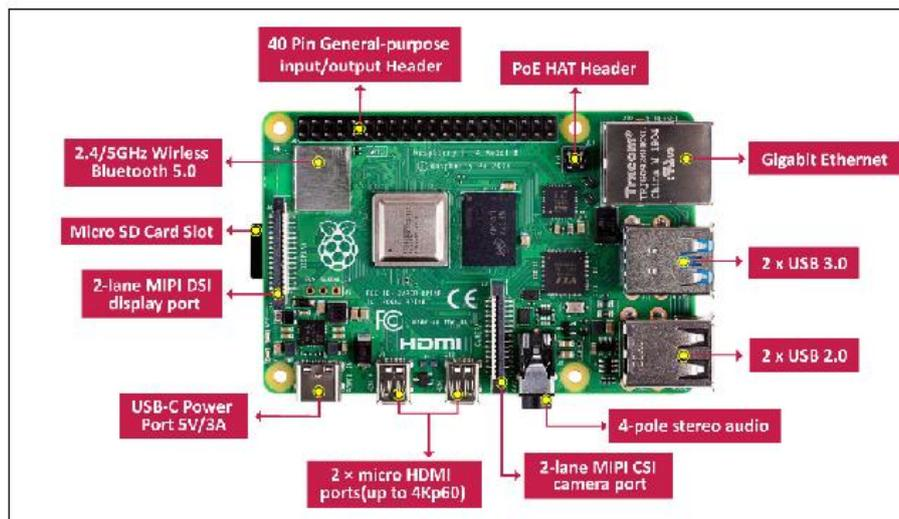
Figure 5. Image of Raspberry Pi circuit
