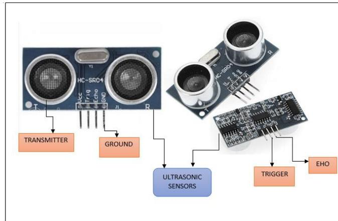
**Figure 2. Ultrasonic Sensor circuit**
