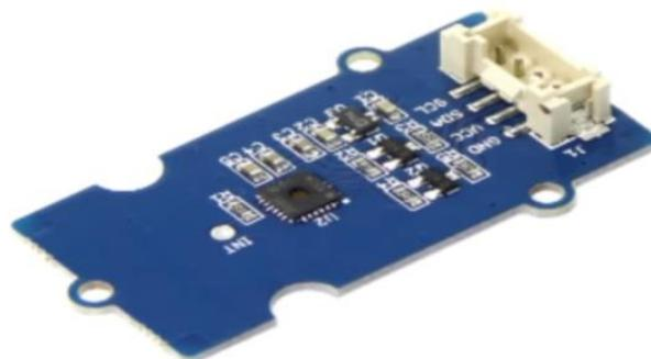
**Figure 3 Grove - Temperature and Humidity Sensor**
