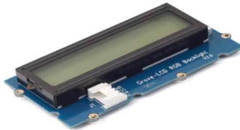
**Figure 7 Grove – LCD RGB Backlighted Display**
