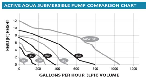
**Figure 15 Head vs. Gallons Per Hour Chart for Pump Determination**
