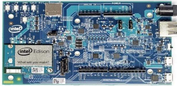
**Figure 1 Intel Edison (In Arduino)**
