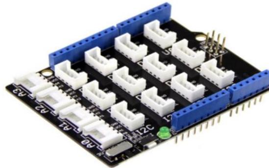
**Figure 2 Base Shield V2**
