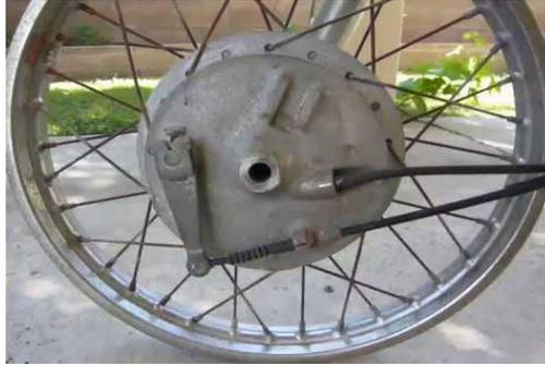
**Figure 1:** Drum brake
