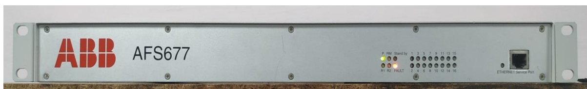
Figure 4: Ethernet switch AFS677 for communication LAN networking
