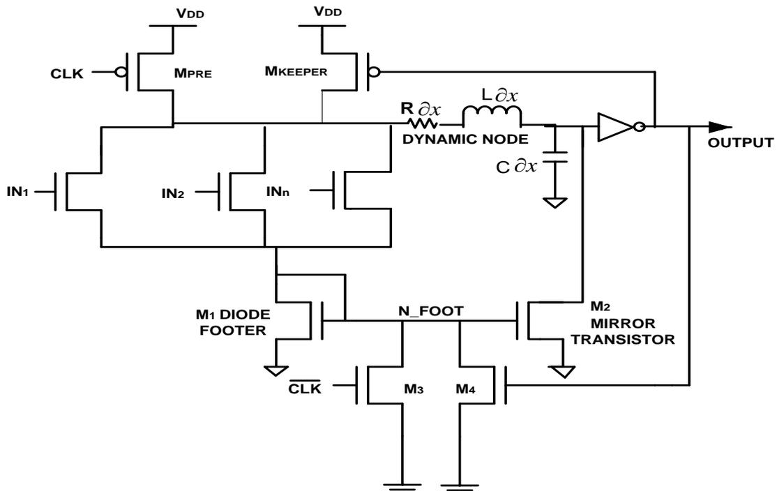
**Fig.7:** Wide OR Gate Using Diode-Footed Domino
