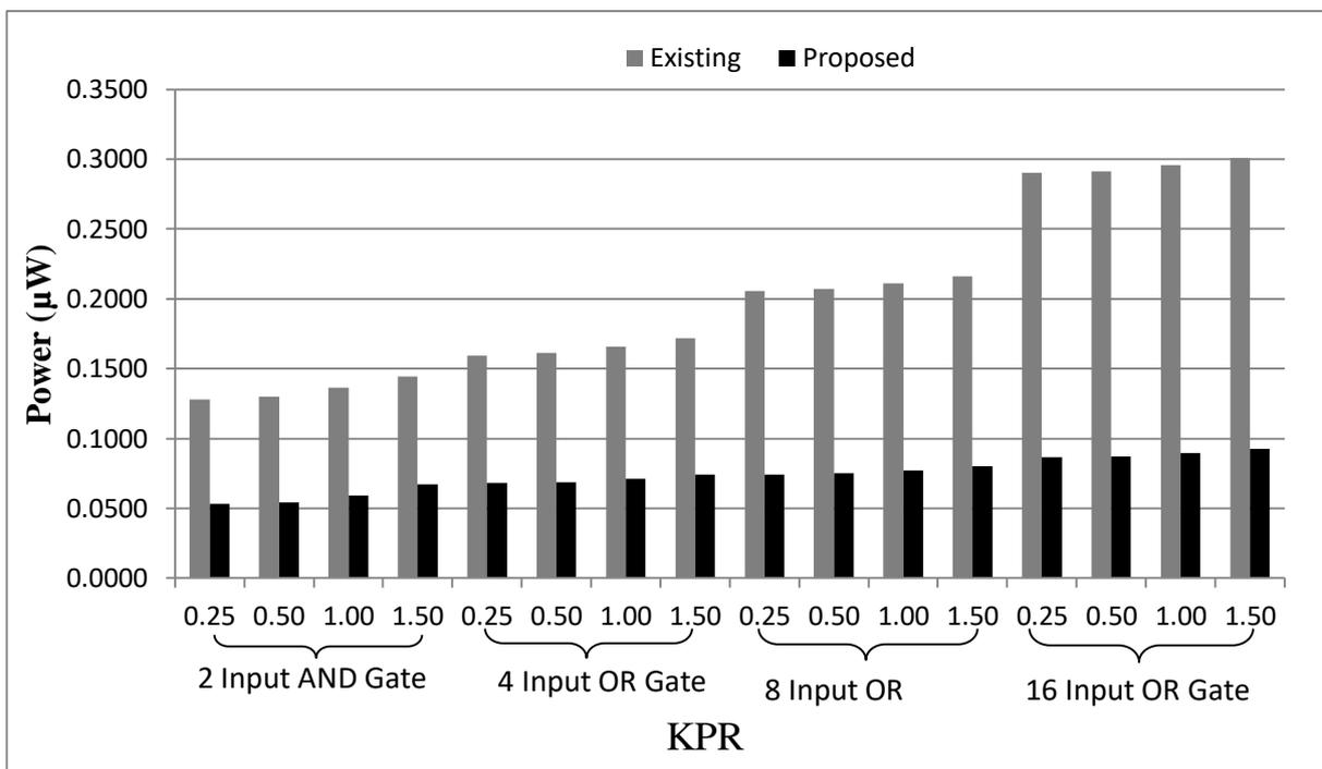
Fig. 11: Comparison of power consumption in existing and proposed circuit with different keeper Ratio (KPR) (n-type: W/L = 1, p-type: W/L = 2)
