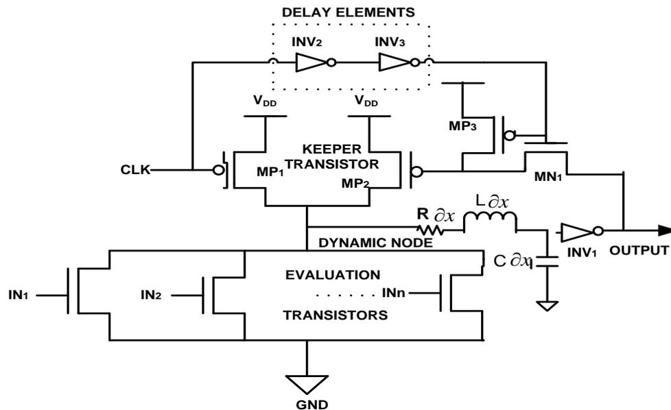
**Fig.5:** High Speed Domino [HSD] Logic Circuit
