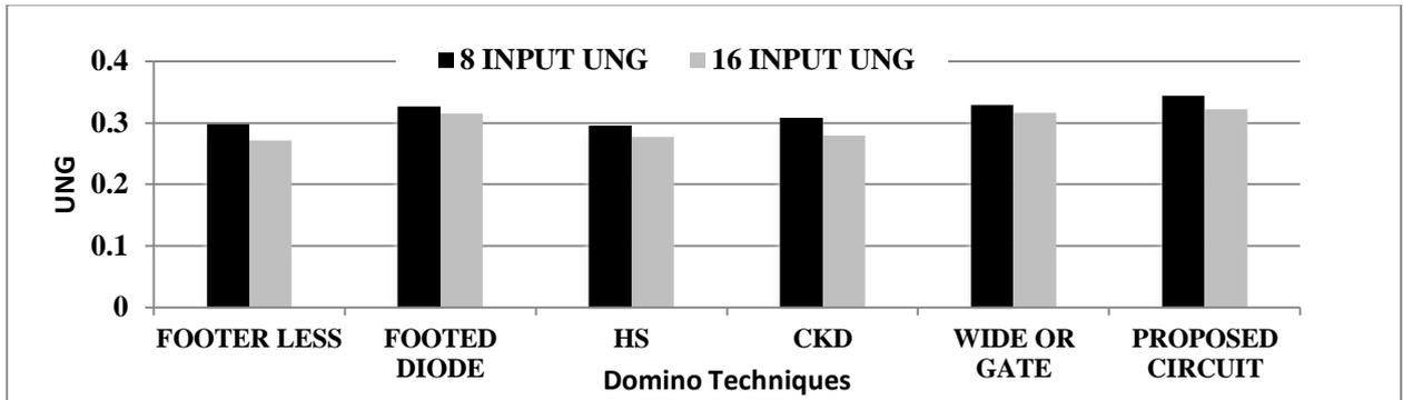
Fig. 10: Comparison of UNG for 8 and 16 inputs OR gate
