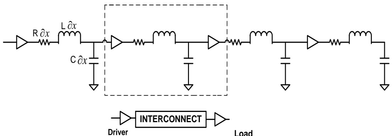
Fig.2. Equivalent Circuit Diagram of RLC Interconnects
