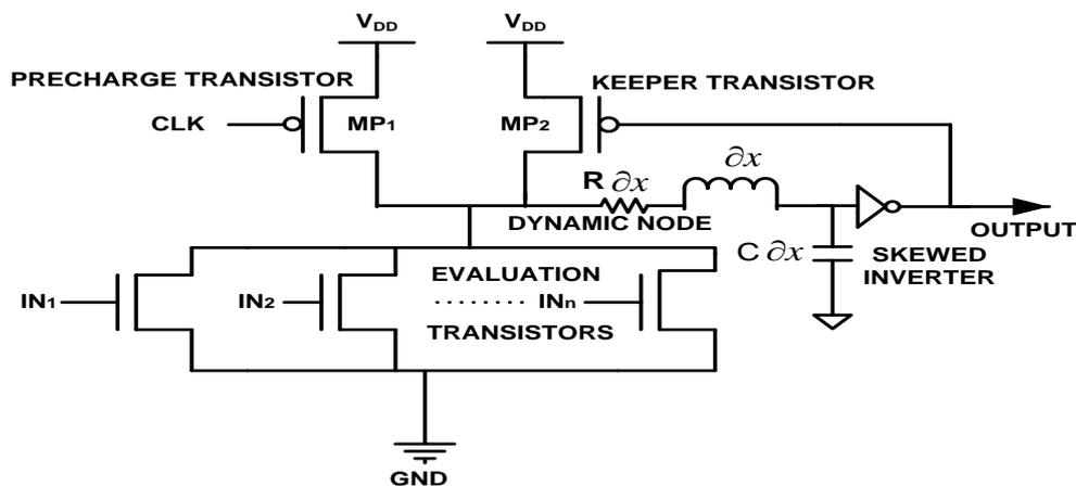
Fig. 3: Conventional High Fan in Domino OR Gate with FooterLess Domino Logic [FLDL]
