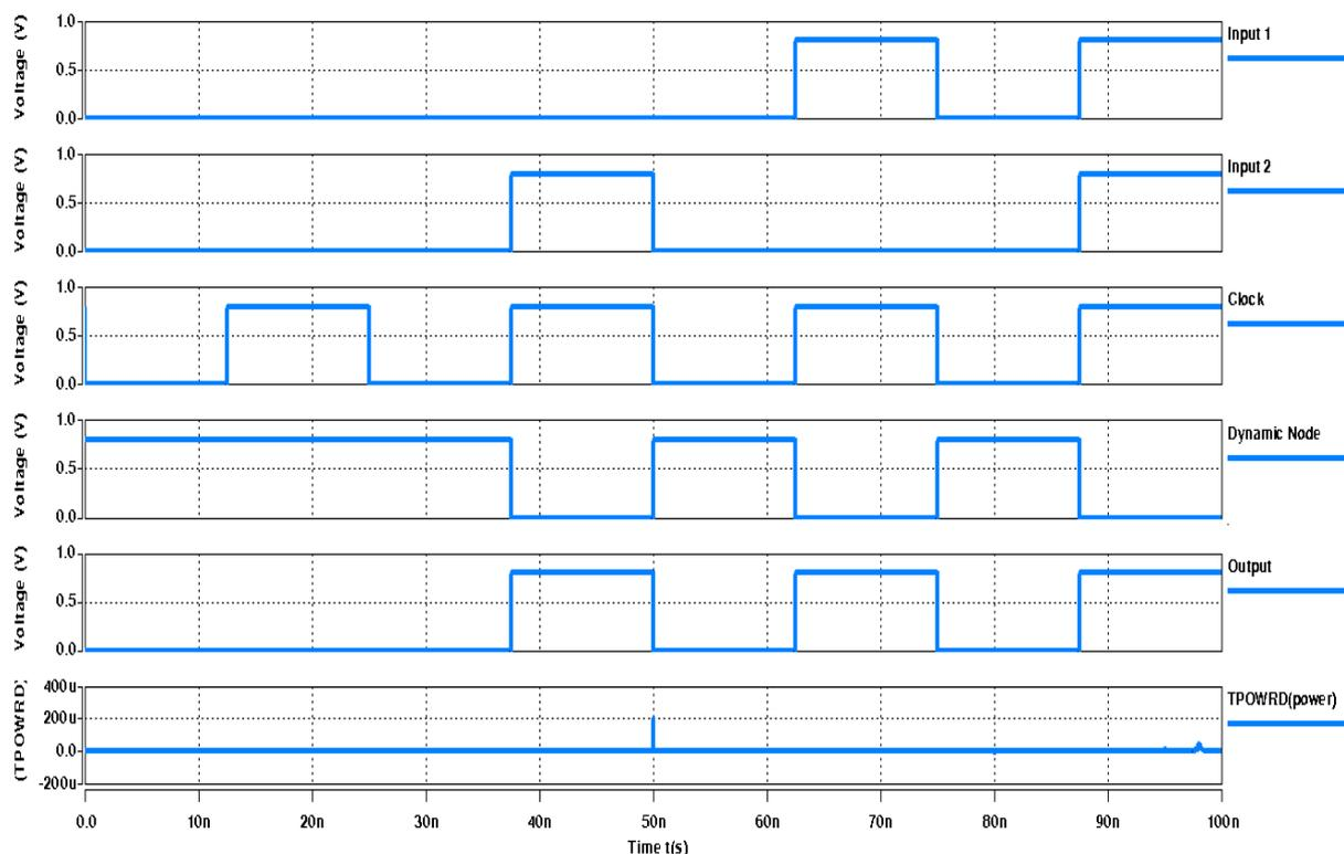
**Fig.9:** Transient characteristics of 2-input ULPS-DPC domino OR gate using HSPICE (the X-axis shows the simulation time in nanosecond and Y-axis shows the voltage in volts) at 10 MHz
