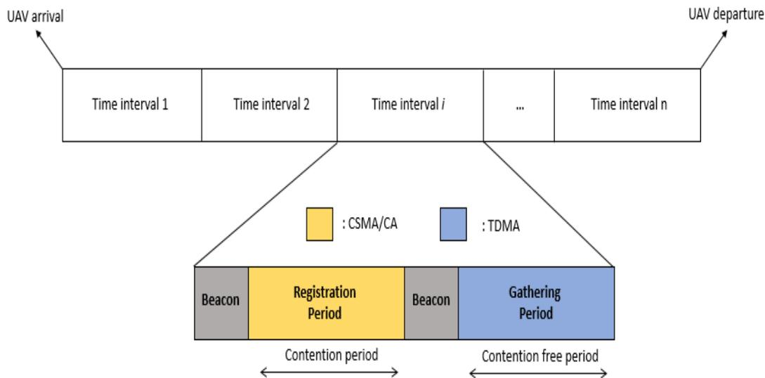
**Figure6:** Time Diagram and Super Frame Of HP-MAC
