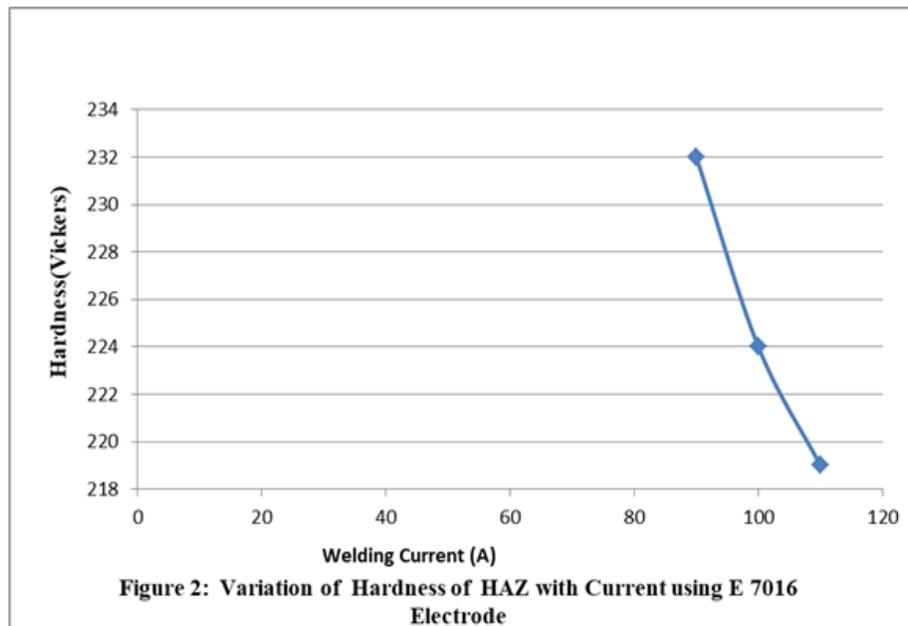
The hardness for heat affected zone for welded plates using electrode E 7016 decreases with increase in current for the whole experimental range as shown in figure 2. At 90 A current the Vickers hardness for
