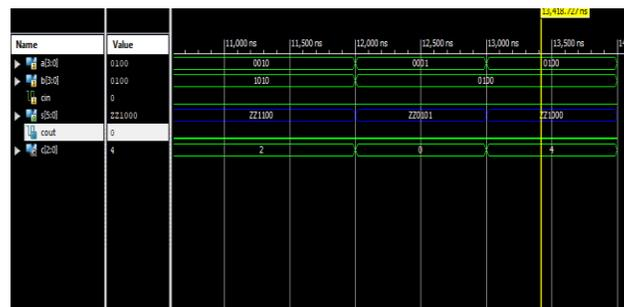
**Figure 5.** output waveform of RCA type 24 – bit adder
