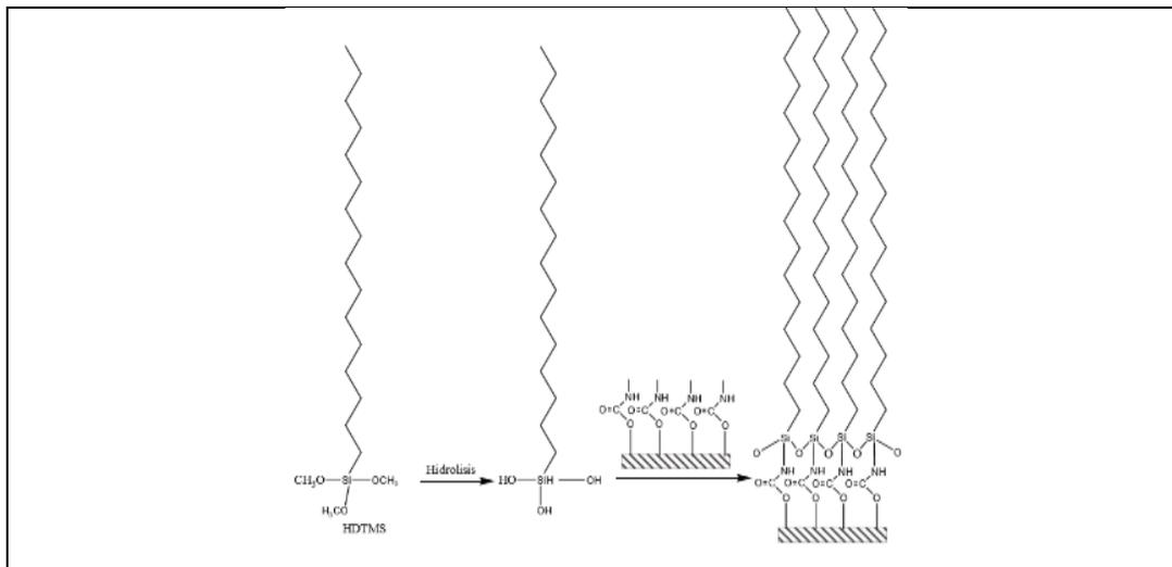
**Figure 3.** The Mechanisms of Hydrophobicity on Spandex by Silane Compounds [18]
