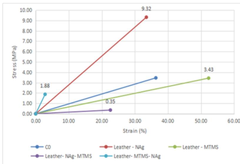
**Figure 5.** The Stress-Strain Curves of Pickle Leather Material
