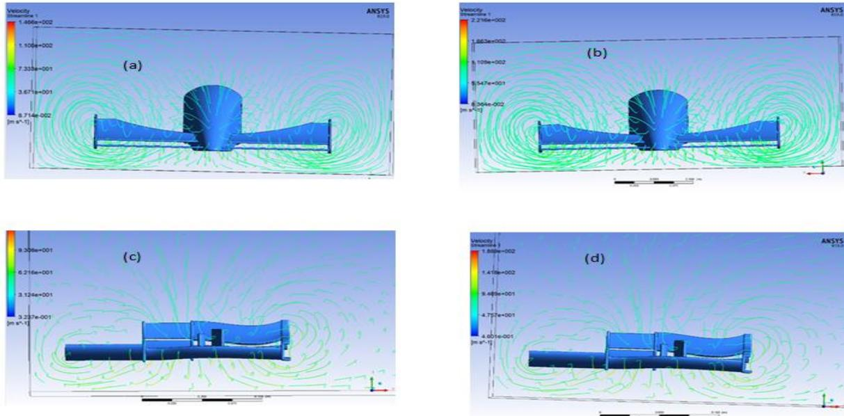
**Figure 7.** (a), (b) shows Velocity contours for McLaren (at 200 and 300 km/hr respectively) and (c), (d) shows the same parameters for Redbull (at 200 and 300 km/hr respectively)
