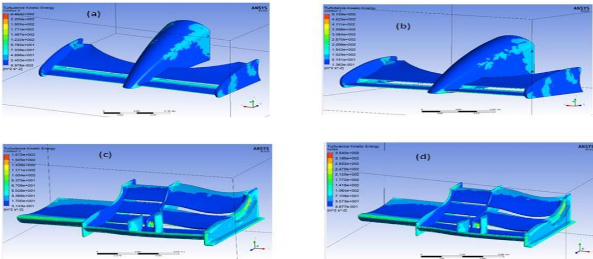
**Figure 6.** (a), (b) shows Turbulent Kinetic Energy contours for McLaren (at 200 and 300 km/hr respectively) and (c), (d) shows the same parameters for Redbull (at 200 and 300 km/hr respectively)
