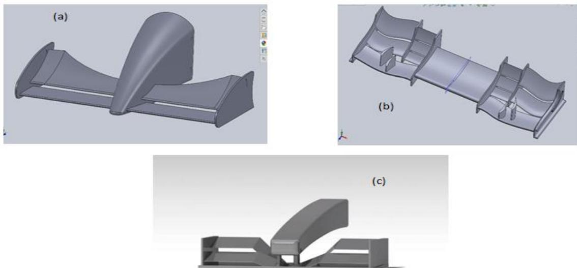
**Fig : 2** (a),(b),(c) shows the 3-D models of McLaren, Redbull and experimental models respectively
