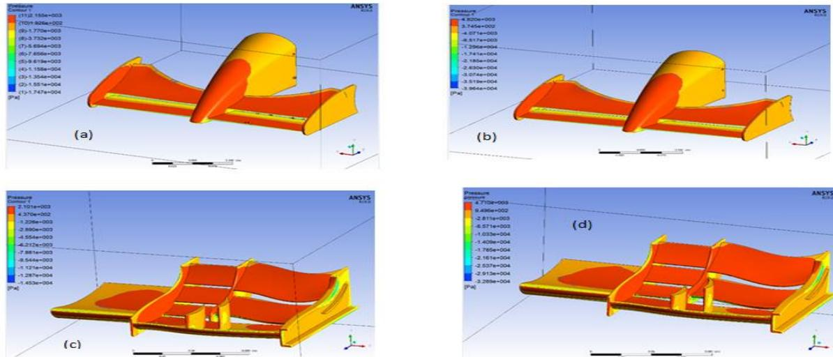
**Figure 5.** (a), (b) shows Pressure contours for McLaren (at 200 and 300 km/hr respectively) and (c), (d) shows the same parameter for Redbull (at 200 and 300 km/hr respectively)
